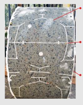
Perforations within internal ring eliminates segregation by controlling and directing concrete flow.
