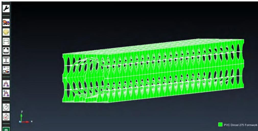
**Figure 22: The geometry of Dincel 275 mm walling panel in GiD environment**
