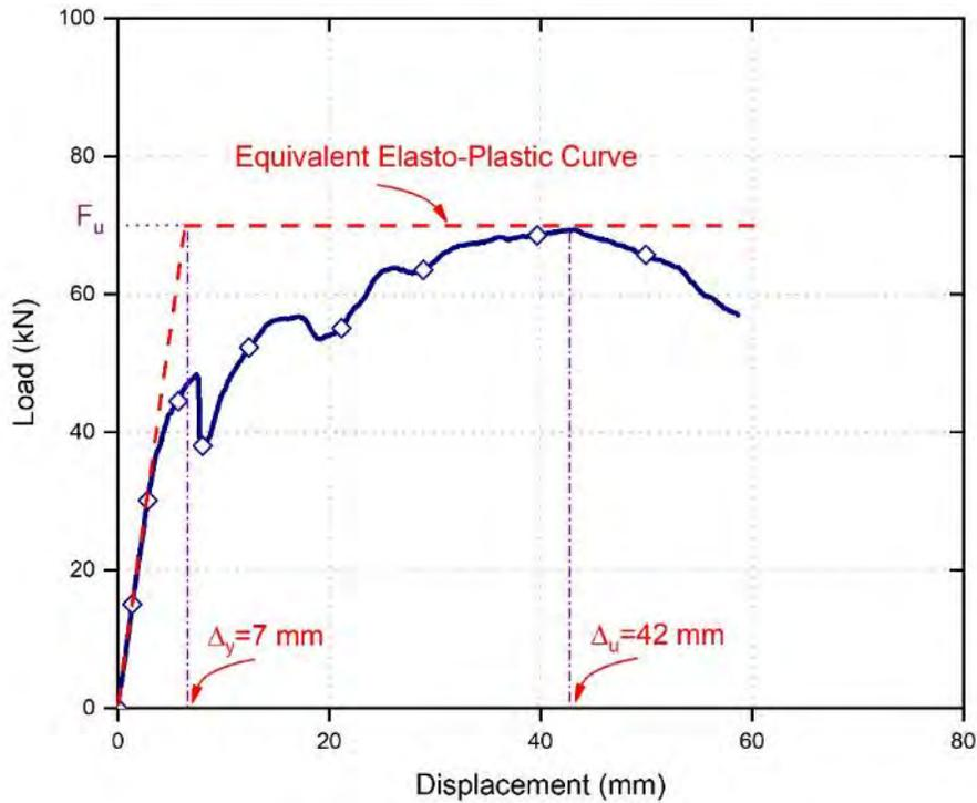
**Figure 18: Finding yield and target displacements for 275 Dintel polymer encased BarChip 48 concrete specimens (average of Samples 1 and 2)**
