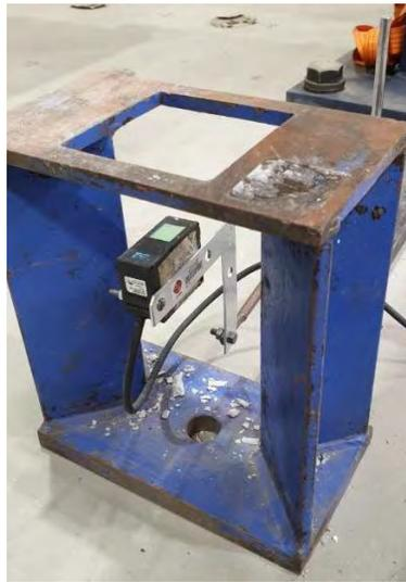
**Figure 6: One of the laser displacement sensors under its protective stand**
