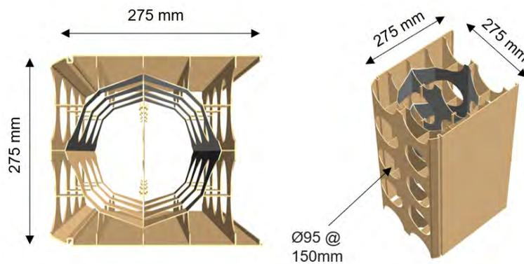
**Figure 5: Three-dimensional views of 275 mm Dintel structural walling panels**
