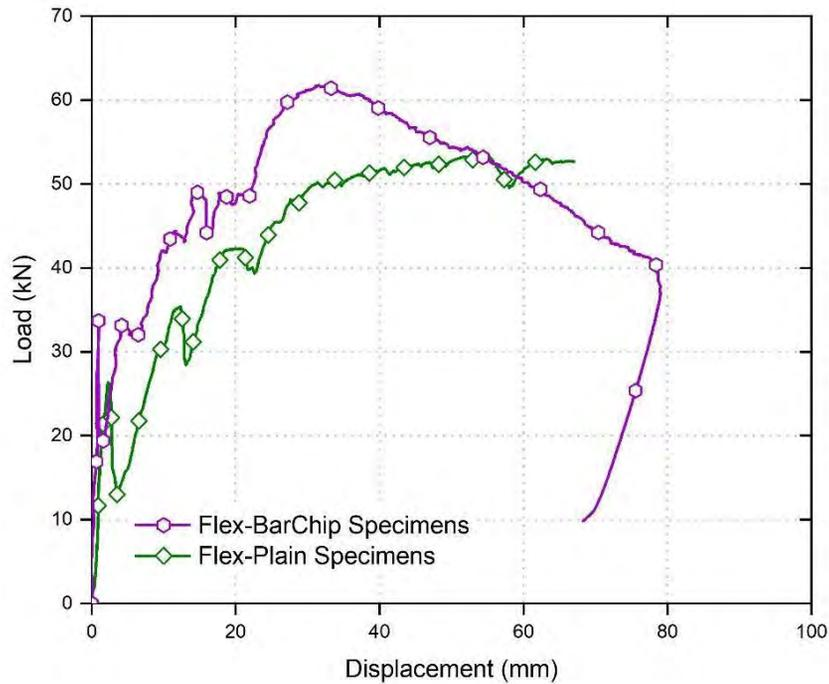
**Figure 14: Comparison between Flex-BarChip and Flex-Plain average load-deflection curves at the age of 24 hours**
