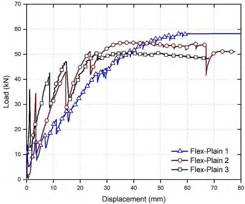
Figure 9: Load-deflection curves for Flex-Plain specimens at the age of 24 hours
