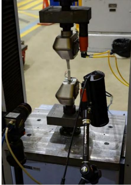
**Figure 4: An overview of the tensile Dintel Polymer testing at the UTS Tech Lab**
