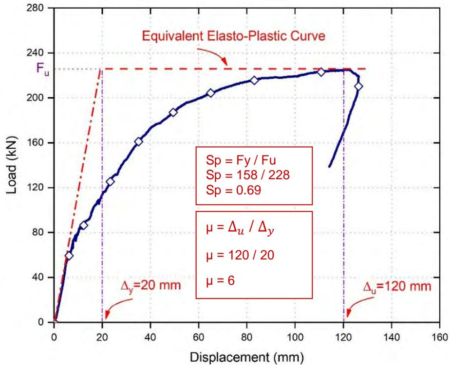
Figure 16: Finding yield and target displacements for 275 Dincel polymer encased reinforced concrete specimens
