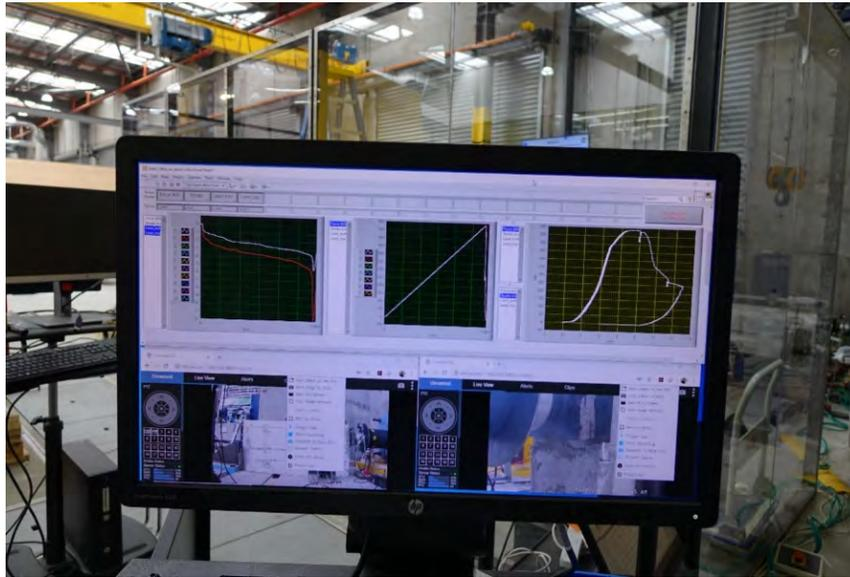
**Figure 8: Closed loop PID Control system (FCS SmartTest One) used for recording and post processing**
