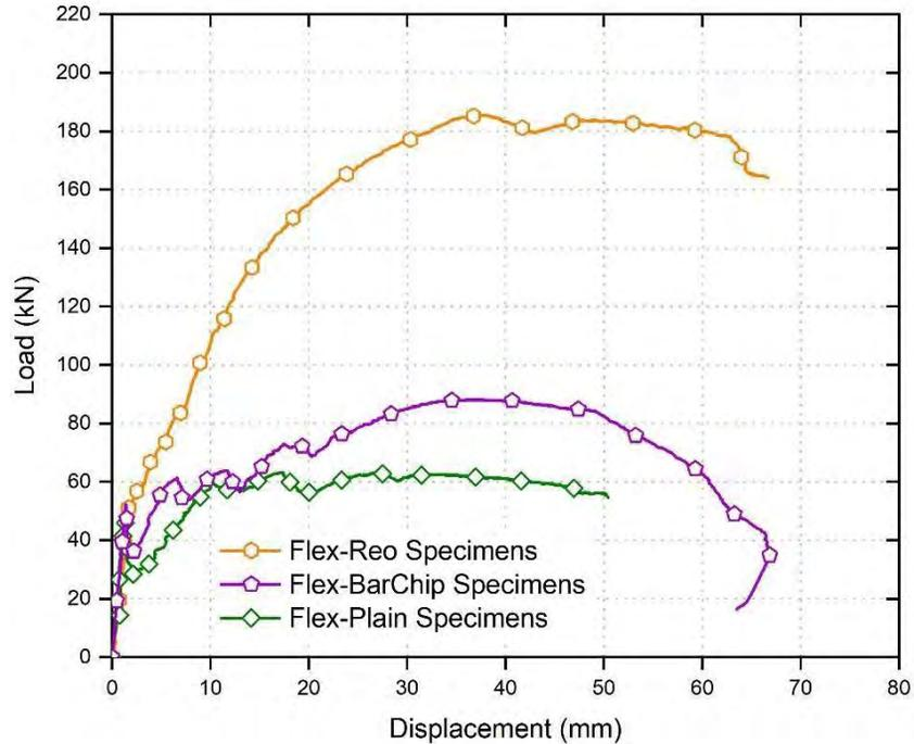
**Figure 15: Comparison between Flex-BarChip, Flex-Plain and Flex-Reo average load-deflection curves at the age of 28 days**
