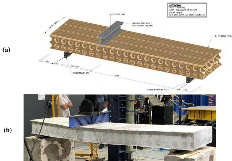
Figure 1: a) Dimensions of the test specimens, b) Overall view of the test specimens
