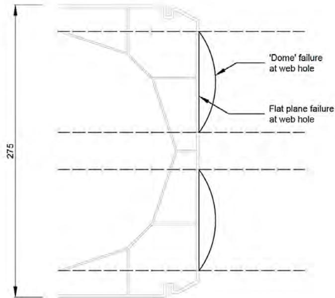
**Figure 13: Illustration of dome shaped failure planes at web holes**
