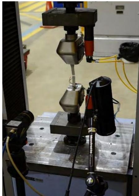
**Figure 4: An overview of the tensile PVC testing at the UTS Tech Lab**
