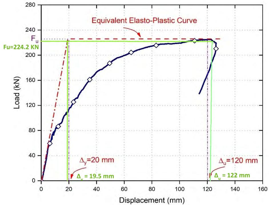
Finding the Yield and Ultimate Displacements for the **BarChip Concrete** specimens:
