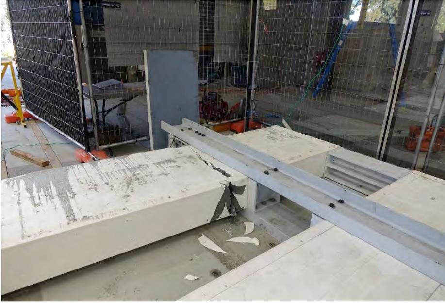
**Figure 10: Failure mode of the walls consisting of plain concrete infill under compressive lateral loads**
