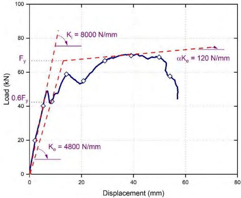
**Figure 21: Finding lateral stiffness values for 275 Dincel encased plain concrete specimens (average of Samples 1 and 2)**
