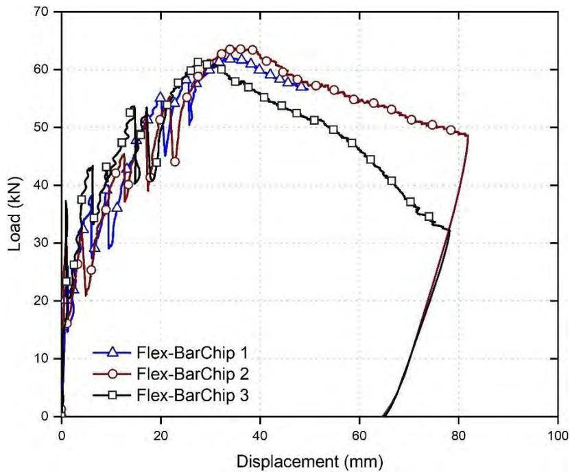
Figure 10: Load-deflection curves for Flex-BarChip specimens at the age of 24 hours
