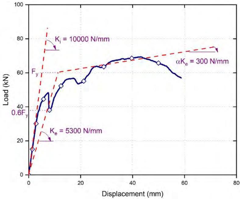
Figure 20. Finding lateral stiffness values for 275 Dintel encased BarChip 48 concrete specimens (average of Samples 1 and 2)
