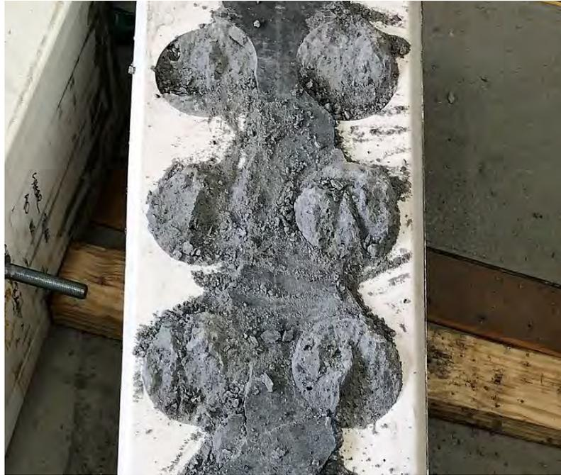
**Figure 12: Dome/conical failure plane observed at web hole locations of Dincel 275 profile**
