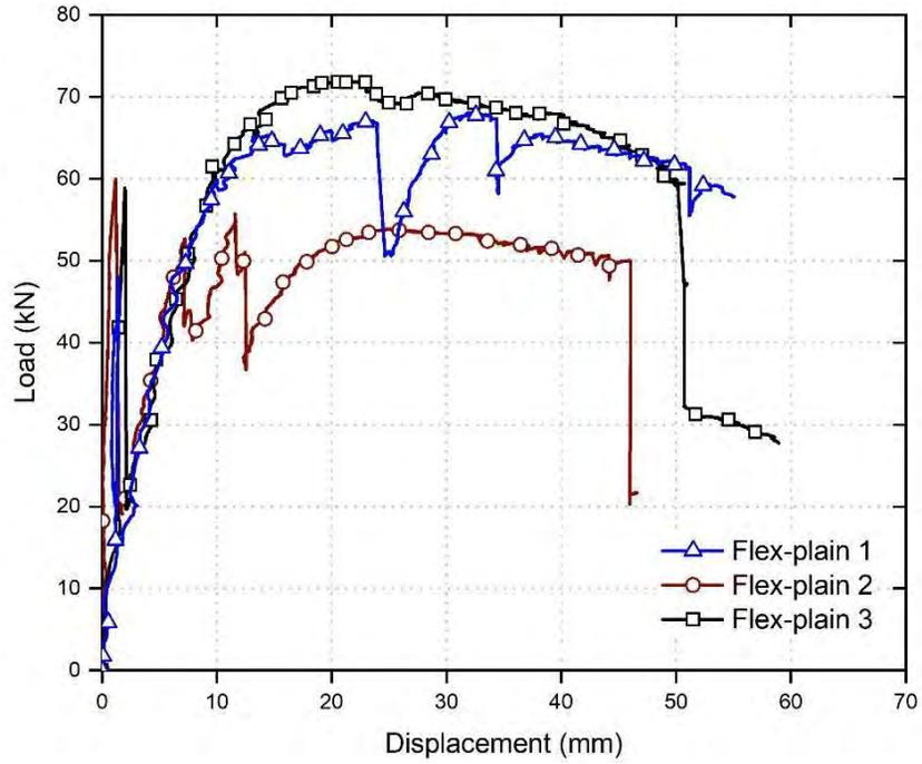
**Figure 11: Load-deflection curves for Flex-Plain specimens at the age of 28 days**
