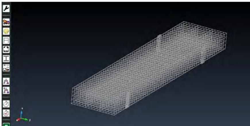
**Figure 26: Mesh settings for specimens in pre-processing software**
