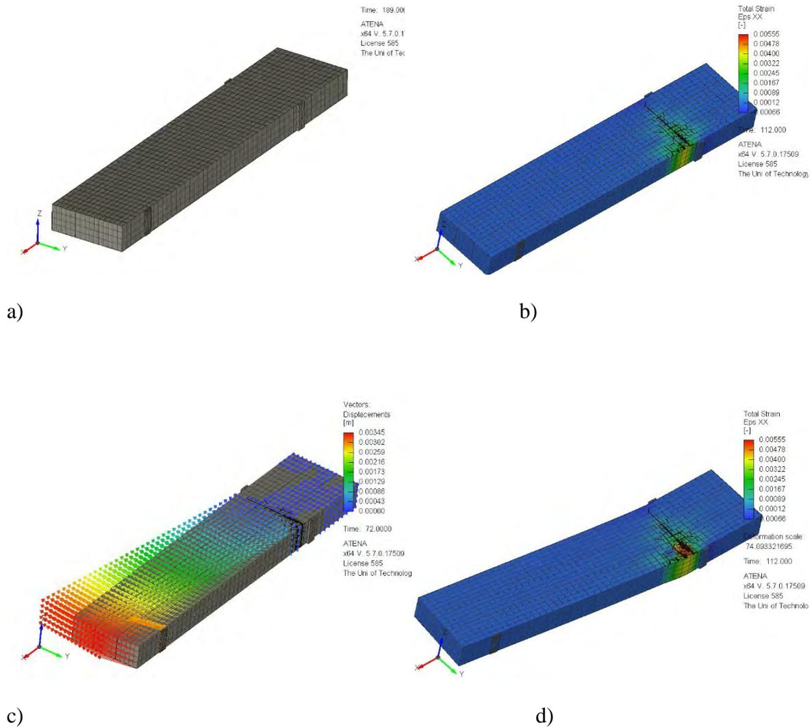
**Figure 27a.** Indicates the geometry of the wall before loading. **Figure 27b** is the crack pattern at the end of the analysis. **Figure 27c** shows the displacement vector. Deformed shape and crack are shown in **Figure 27d**.
