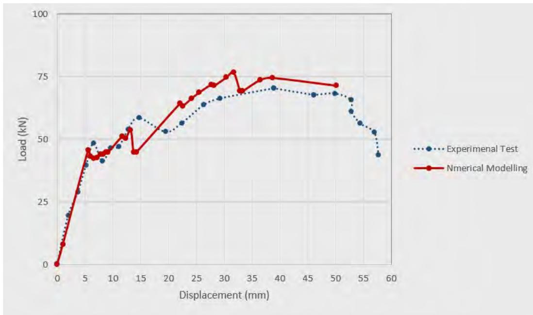
**Figure 28: Load-deflection curve to compare the lateral stiffness values for 275 Dincel Polymer encased plain concrete specimens by both experiment and FEM analysis**
