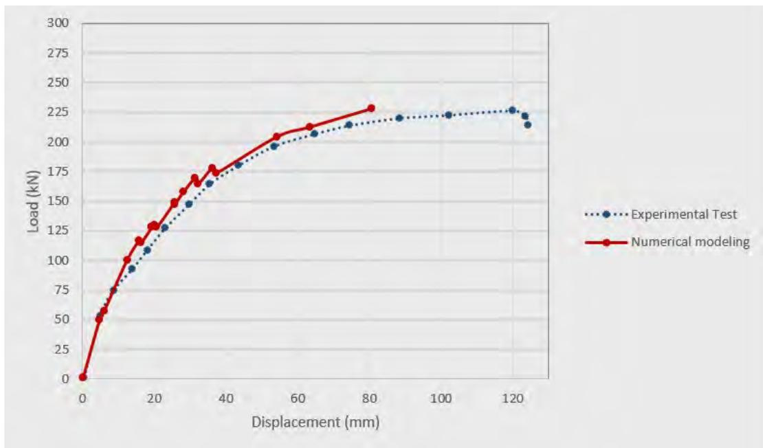
**Figure 30: Load-deflection curve to compare the lateral stiffness values for 275 Dintel encased reinforced concrete specimens by both experiment and FEM analysis**
