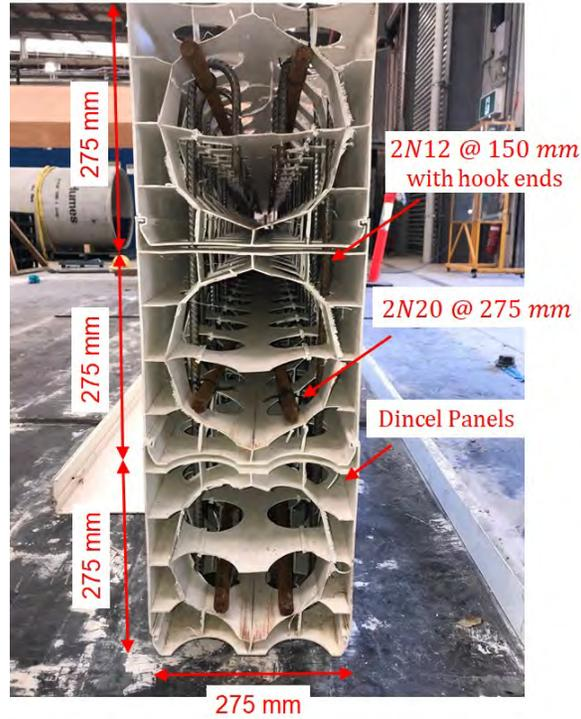
**Figure 4: Front view of a Dintel Polymer encased wall with steel reinforcements**
