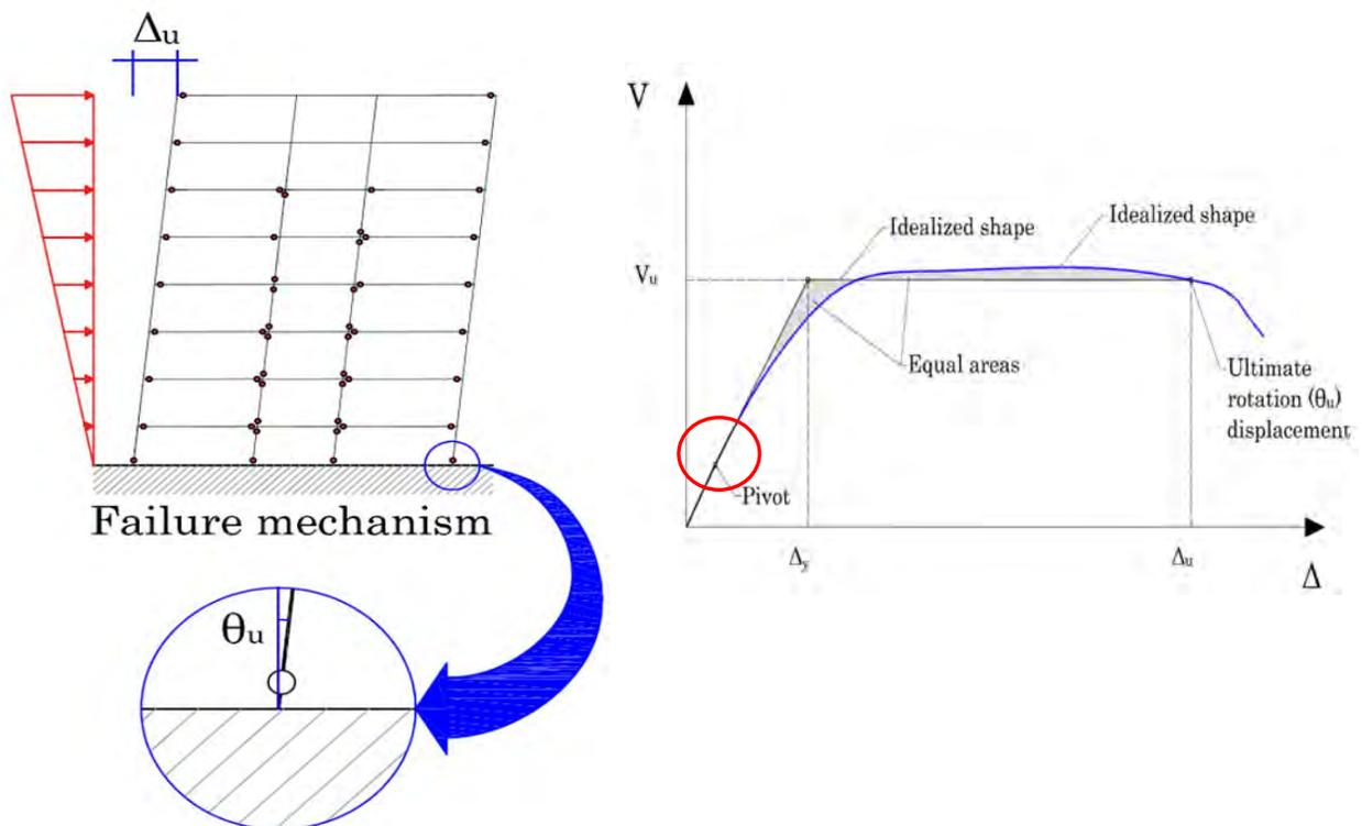
Figure A1.1 Ultimate Rotation and Pivot Point defined in the Proposed Model
