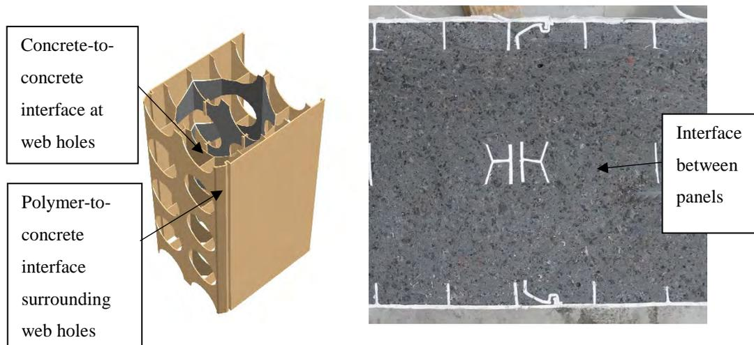
**Figure 11: Dincel panel interface (left), cut test specimen showing interface (right)**
