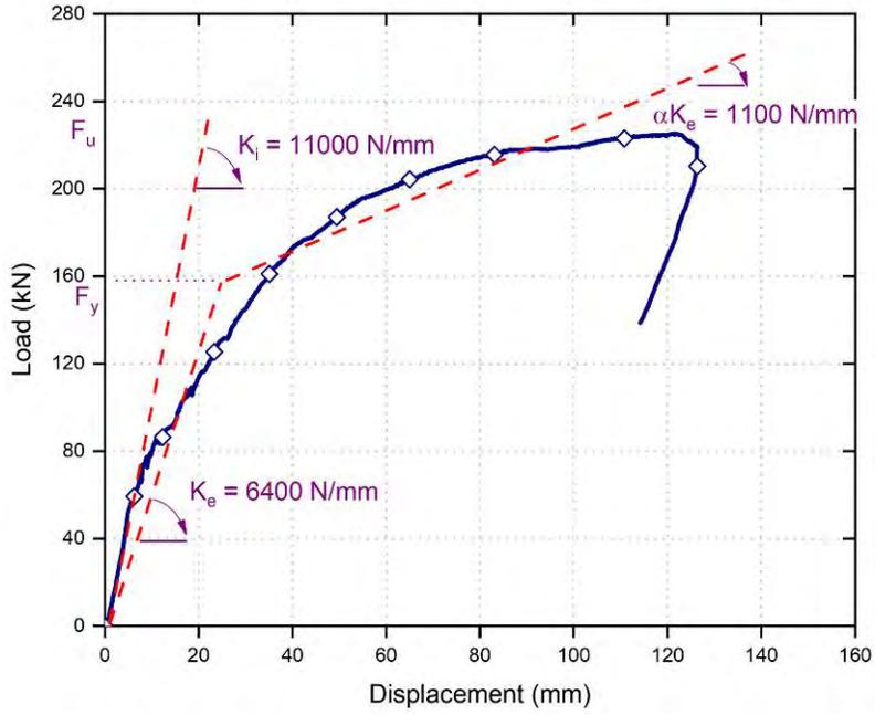
Figure 19: Finding lateral stiffness values for 275 Dintel encased reinforced concrete specimens (average of Samples 1 and 2)
