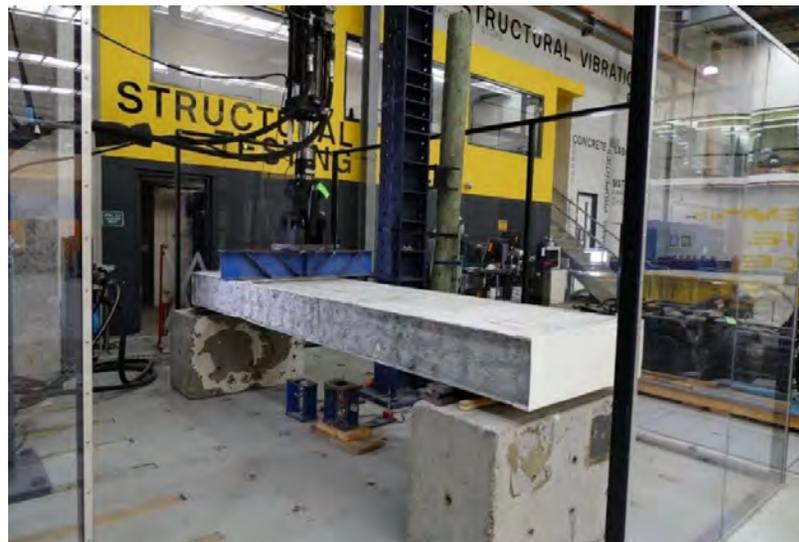
**Figure 5: Three-point bending test configuration**
