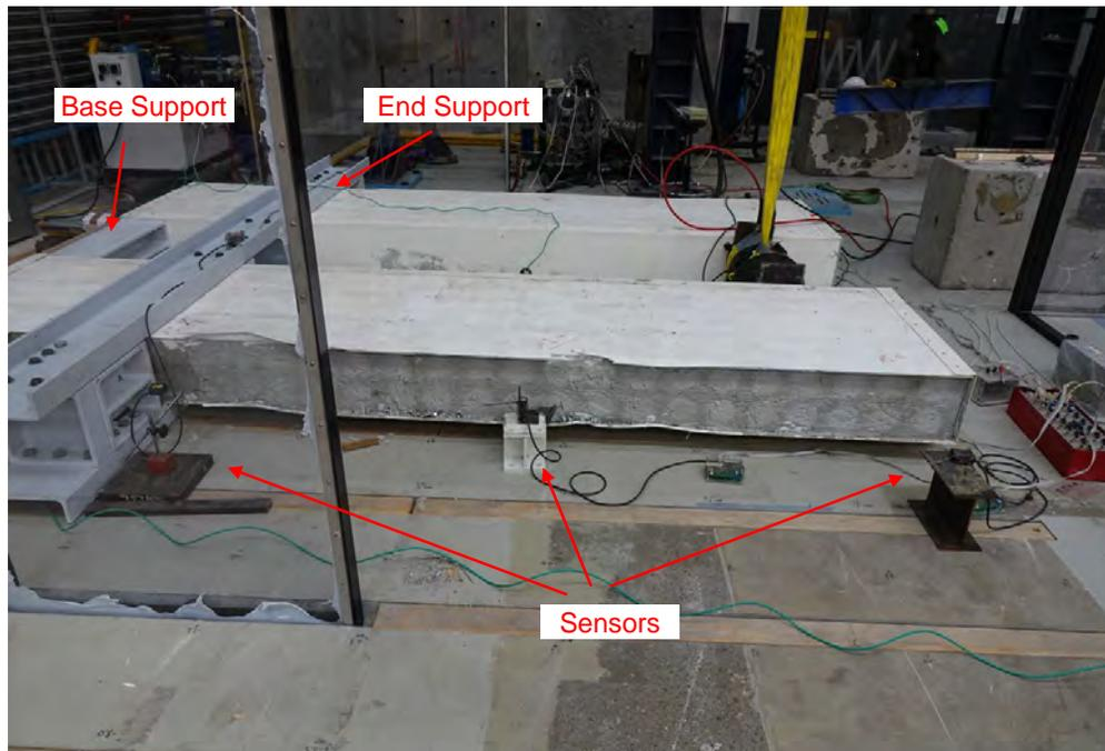
**Figure 3: Base and end supports in 275 Dintel structural walling panels**
