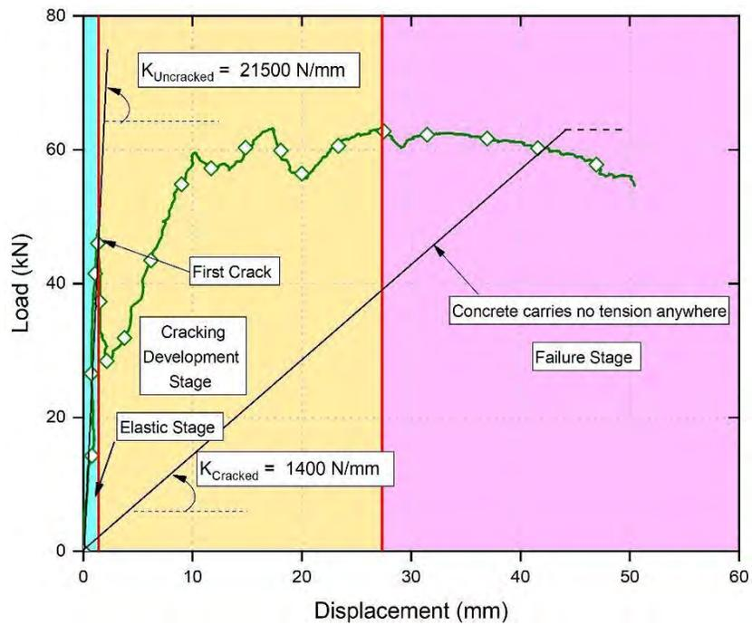
**Figure 18: Stiffness calculation for Flex-Plain specimens**
