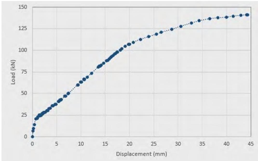
**Figure 31: Load-deflection curve for conventional 270 mm thick reinforced wall (without 275 Dintel) subjected to lateral load by FEM analysis.**
