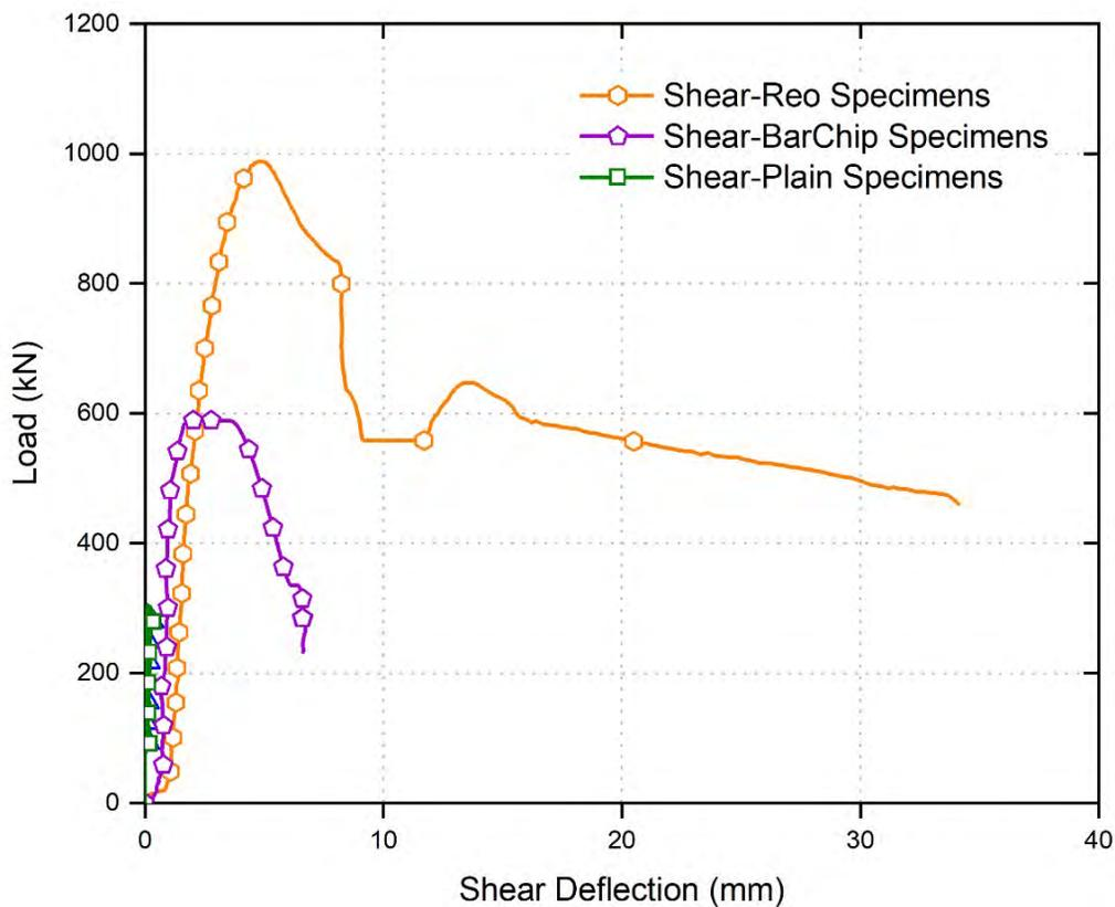
**Figure 10: Average load-shear deflection curves obtained from direct shear tests**
