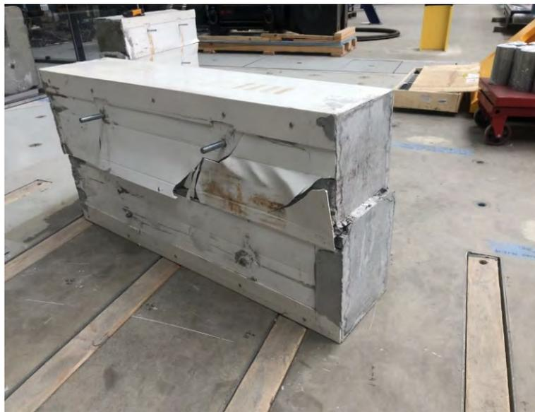
**Figure 9: Failure of one of the test specimen after reaching the maximum shear capacity at the interface of composite Dintel Polymer encased 275 mm Dintel structural walling panels**
