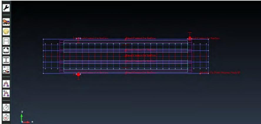
**Figure 25: Assigning load point and support boundary conditions**
