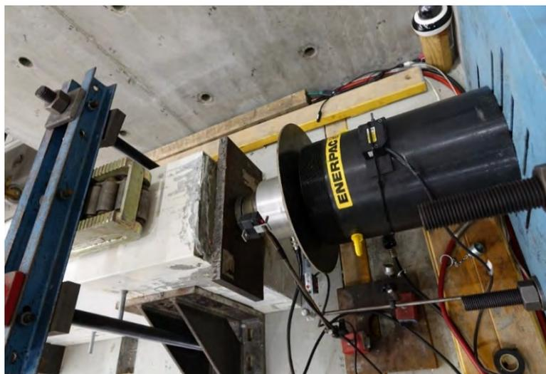
**Figure 7: Hydraulic cylinder used in experimental study to apply horizontal load**
