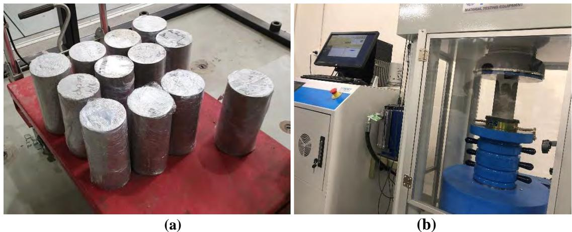
Figure 2: Concrete compression cylinder tests; a) Samples taken from the fresh concrete mix, b) Concrete compression test in process at UTS Tech Lab
