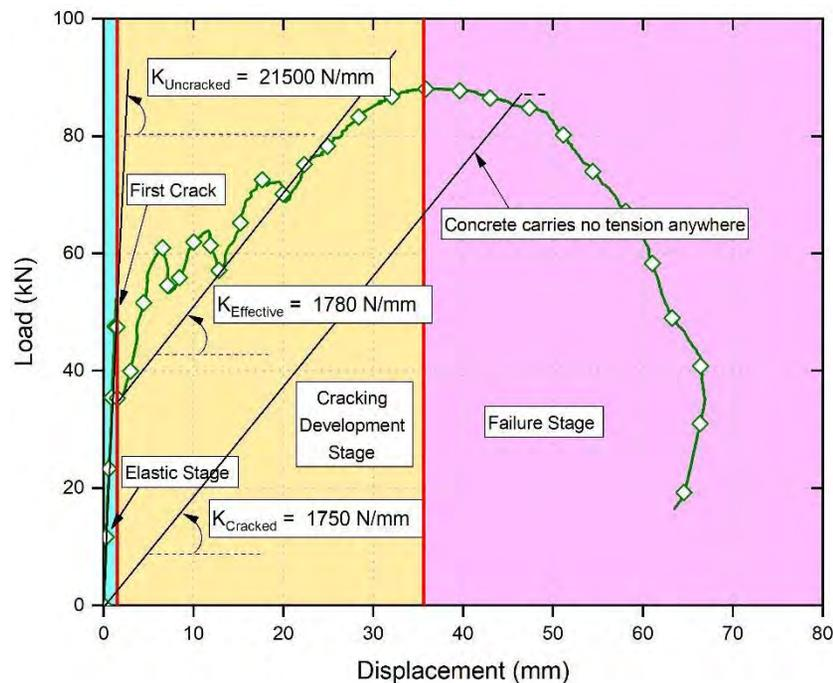
Figure 16: Stiffness calculation for Flex-BarChip specimens
