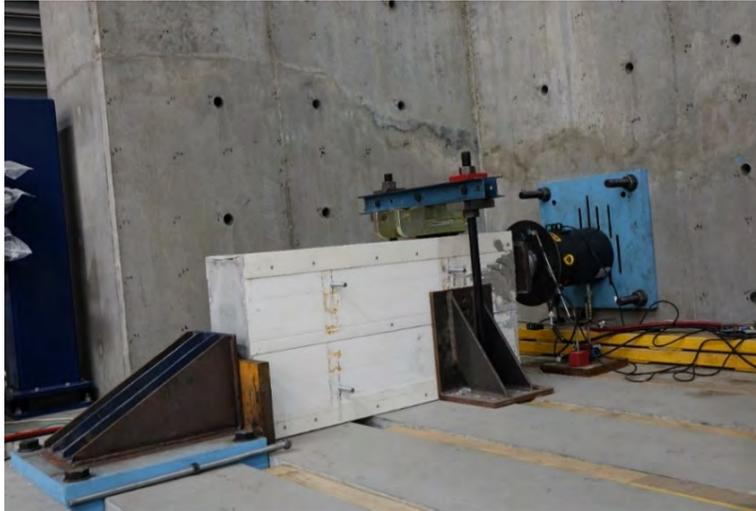
**Figure 6: An overview of the direct shear test configuration at the Tech Lab**
