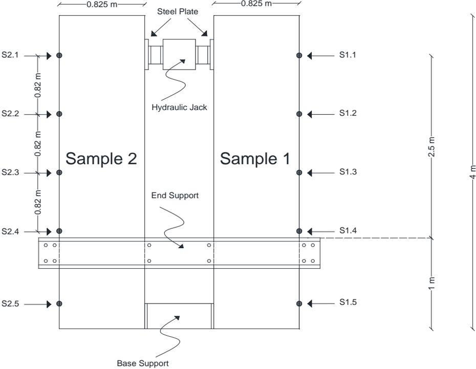
**Figure 1: Schematic diagram of pushover test setup (S illustrates sensors)**
