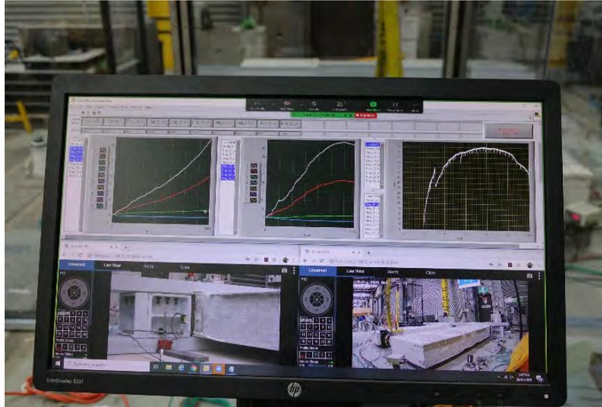
**Figure 9: Data acquisition system used in the experimental study**
