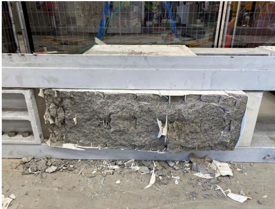
**Figure 11: Section of specimen consisting of plain concrete infill at failure plane**
