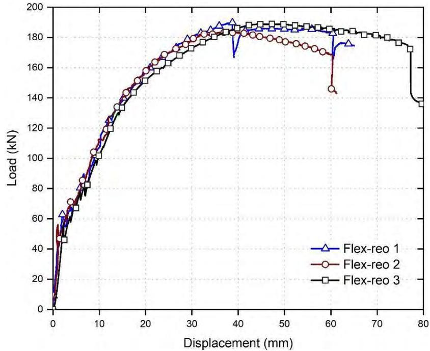
**Figure 13: Load-deflection curves for Flex-Reo specimens at the age of 28 days**
