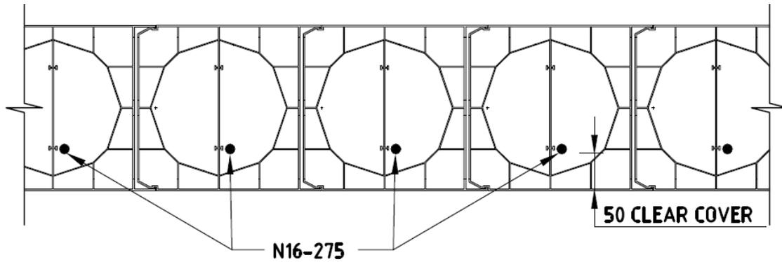
Where more capacity is required, 275 Dincel with N16, N20, or N24 longitudinal reinforcement bars at 275mm centres (Dincel webs work as crack inducers/controllers, hence horizontal steel for crack control purposes is not required) can also be used in any harsh environment for the following reasons:
