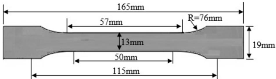
**Figure 3: Dog-bone coupon specimens prepared for tensile tests according to ASTM D638**
