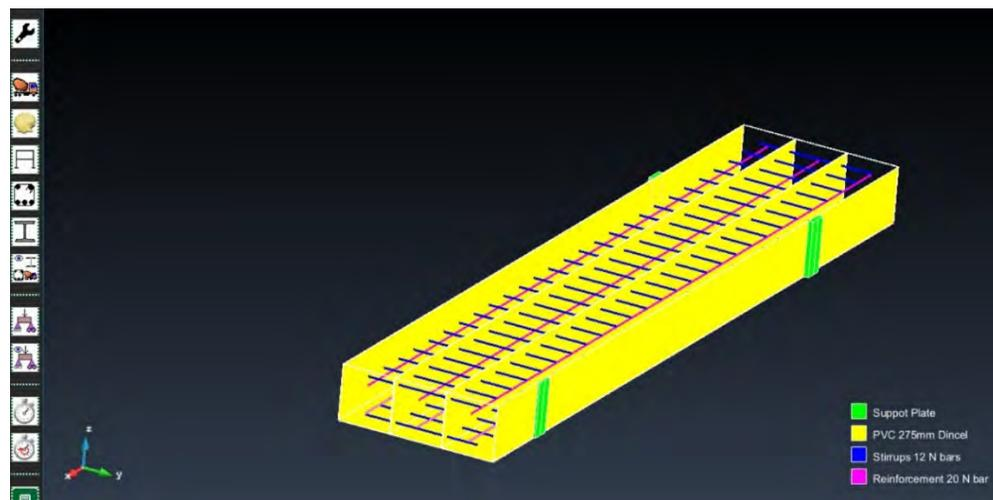
**Figure 24: Defining different materials and reinforcement bars positions**
