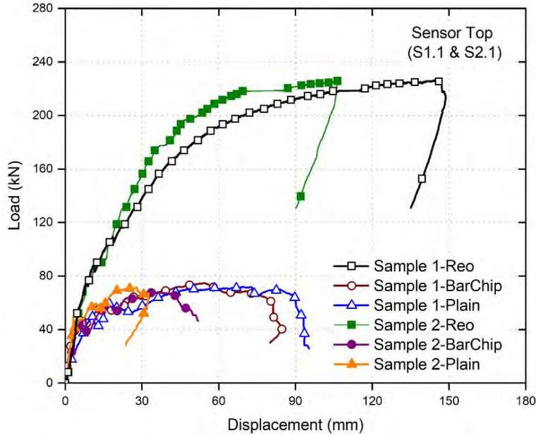
**Figure 15: Average load-displacement curves measured by top sensors in Samples 1 and 2 for all specimens**
