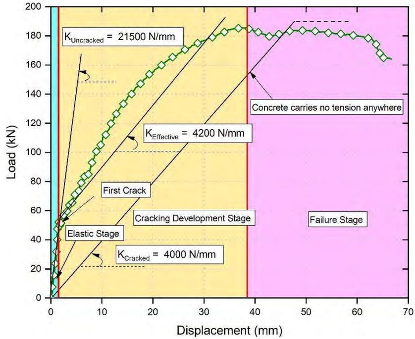
**Figure 17: Stiffness calculation for Flex-Reo specimens**
