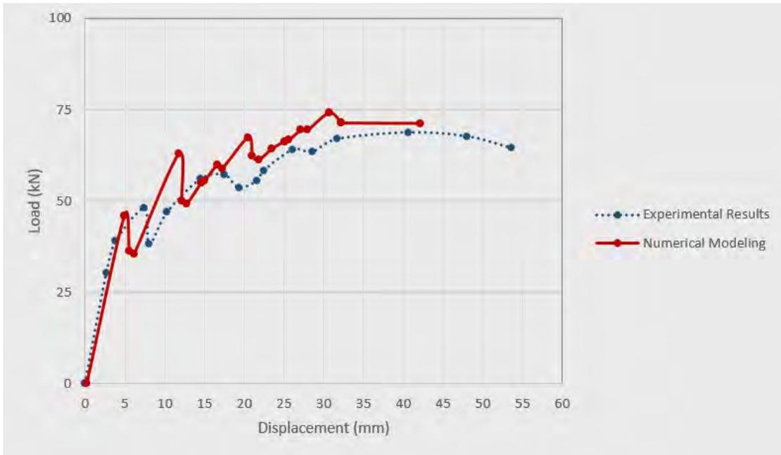
**Figure 29: Load-deflection curve to compare the lateral stiffness values for 275 Dintel encased BarChip concrete specimens by both experiment and FEM analysis**
