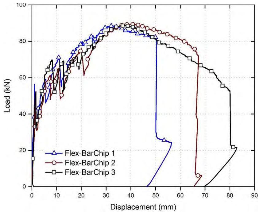
**Figure 12: Load-deflection curves for Flex-BarChip specimens at the age of 28 days**
