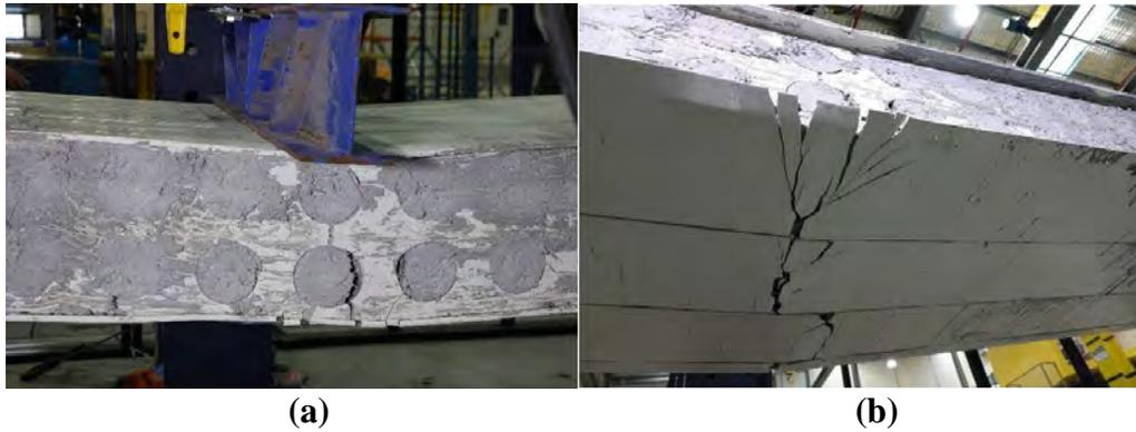
**Figure 8: Failure of one of the BarChip 48 fibre reinforced concrete specimens after reaching the maximum bending moment capacity; a) Front side cracks, b) Underside cracks**
