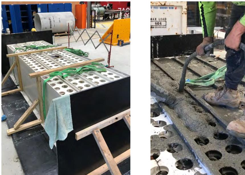
**Figure 7. Placement and vibration of concrete within Dincel panels orientated horizontally**
