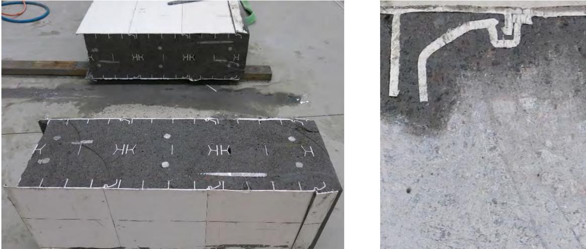
**Figure 8. Cut Dintel specimen demonstrating adequate concrete compaction**
