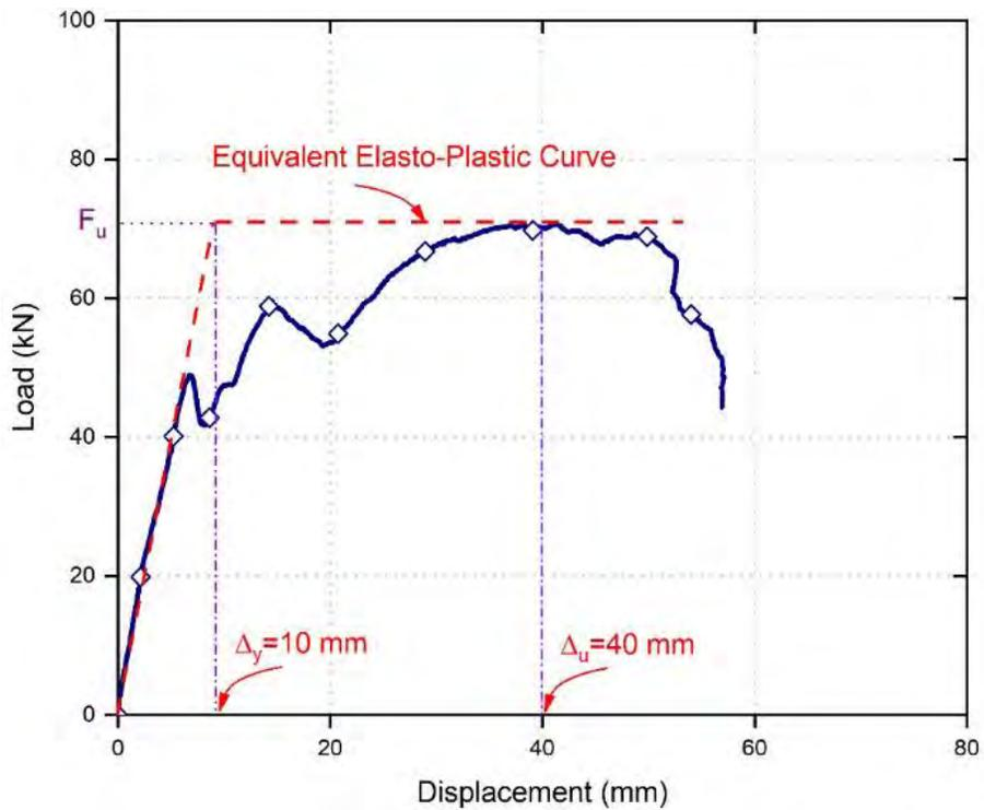
Figure 17: Finding yield and target displacements for 275 Dincel polymer encased plain concrete specimens
