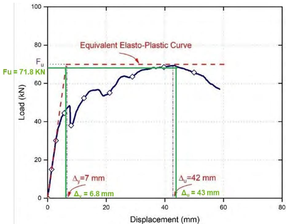
Finding the Yield and Ultimate Displacements for the **Plain Concrete** specimens:
