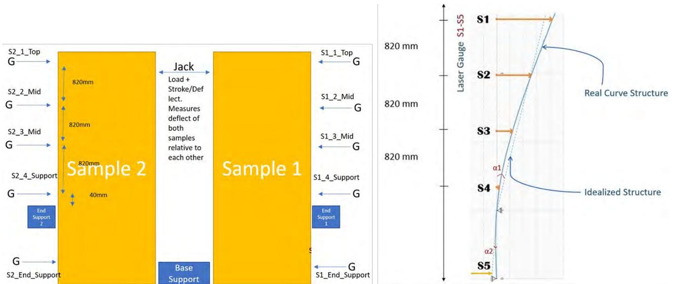
Figure A1.2 Test setup and idealized structure
