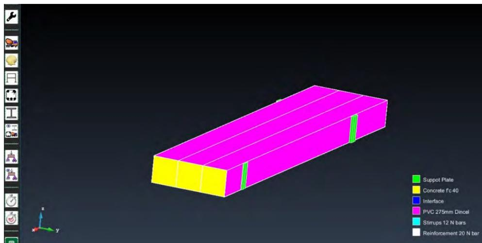
**Figure 23: Defining different materials for specimens**
