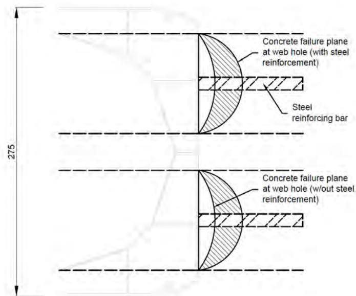
**Figure 14: Illustration of dome shaped failure planes at web holes with steel reinforcement**
