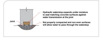
FIGURE 1 - HYDROPHILIC WATERSTOP AT WALL TO SLAB/FOOTING JOINT
