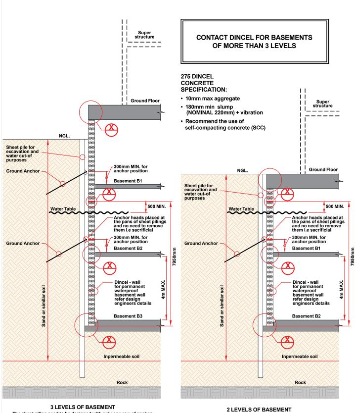
The sheet piling need to be designed with only one row of anchor points if the second row of anchors shown are below the water table, unless second row of anchors and sheet piling are sacrificial. 2 LEVELS OF BASEMENT The sheet piling need to be designed with only one row of anchor points.
