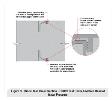
The Dincel panel joints at both faces form very tight joints when they snap-connect to each other. The joints' tightness is further increased when the panels receive concrete infill. The concrete slurry consists of cement and water which further seals the snapped joints. In addition to all this, autogenous healing of the concrete slurry also occurs at the snapped joints where the barbs are located. As a result, a waterproof\* Dincel Wall is achieved as proven by the testing to date.
