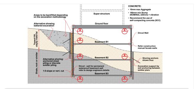
Figure 4 - Basement Construction For Permanent Or Tidal Water Table Below Footing Invert Level
