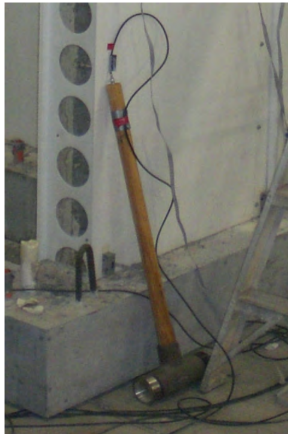
Fig 4.9 - The 12 lb Modal Hammer used for hammer tests
