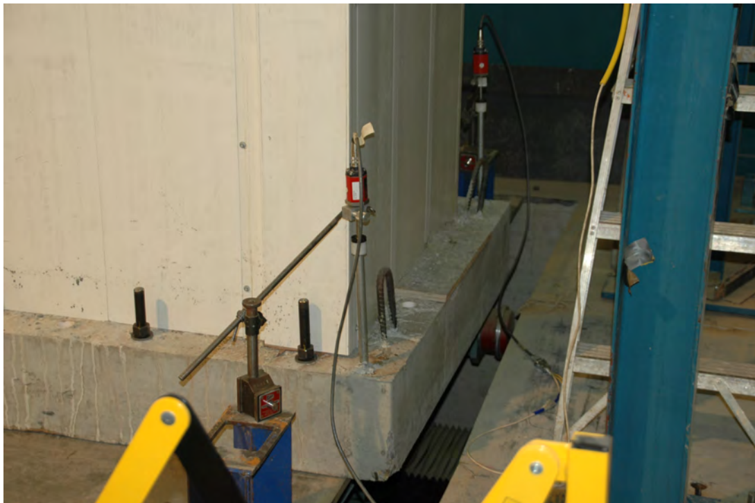
Fig 4.5 –Unreinforced Wall unit and base on UTS shake table prior to testing
