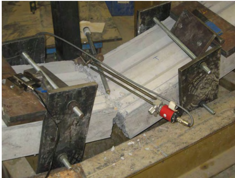
Fig 6.5 - Conventional Reinforced Concrete Beam Specimen after failure
