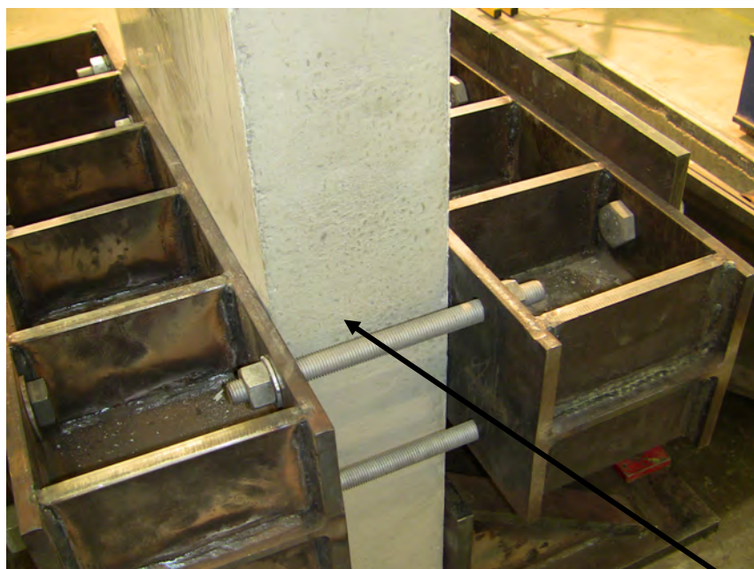
Figure 5.14 (b) Dincel Sample Crack at X = 700mm
