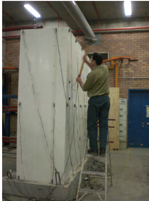
Fig 4.10 – Conducting Hammer Test on the specimen
