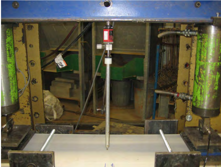
Fig 6.1 – Linear variable displacement transducer (LVDT) measuring displacement at mid span of the beam
