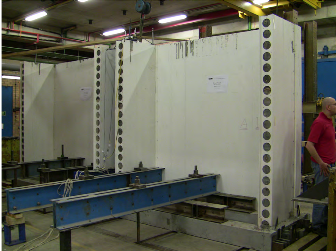
Figure 4.8 – Dintel Wall footing connection to strong floor
