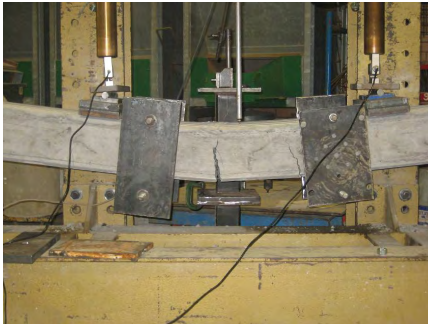
Fig 6.4 – Large flexural cracks developing in Conventional Reinforced Concrete Beam Specimen
