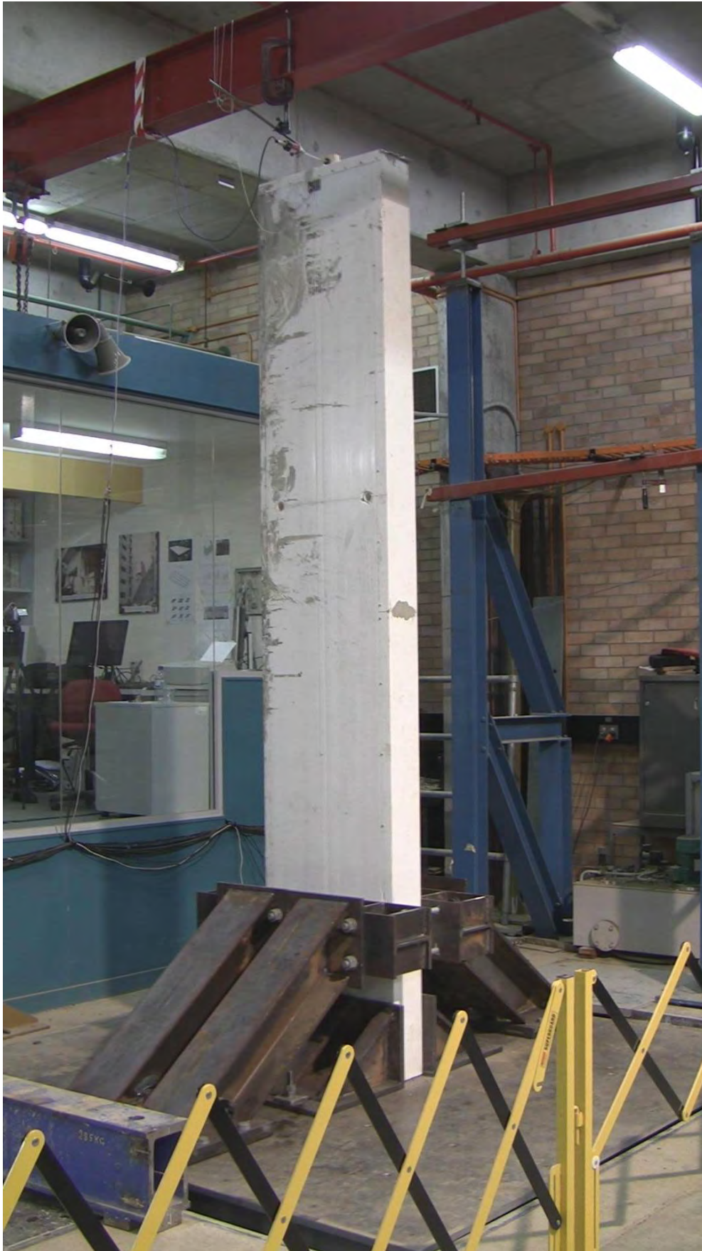
Fig 5.8 – Dincel System Sample 'C' set up on UTS Shake Table
