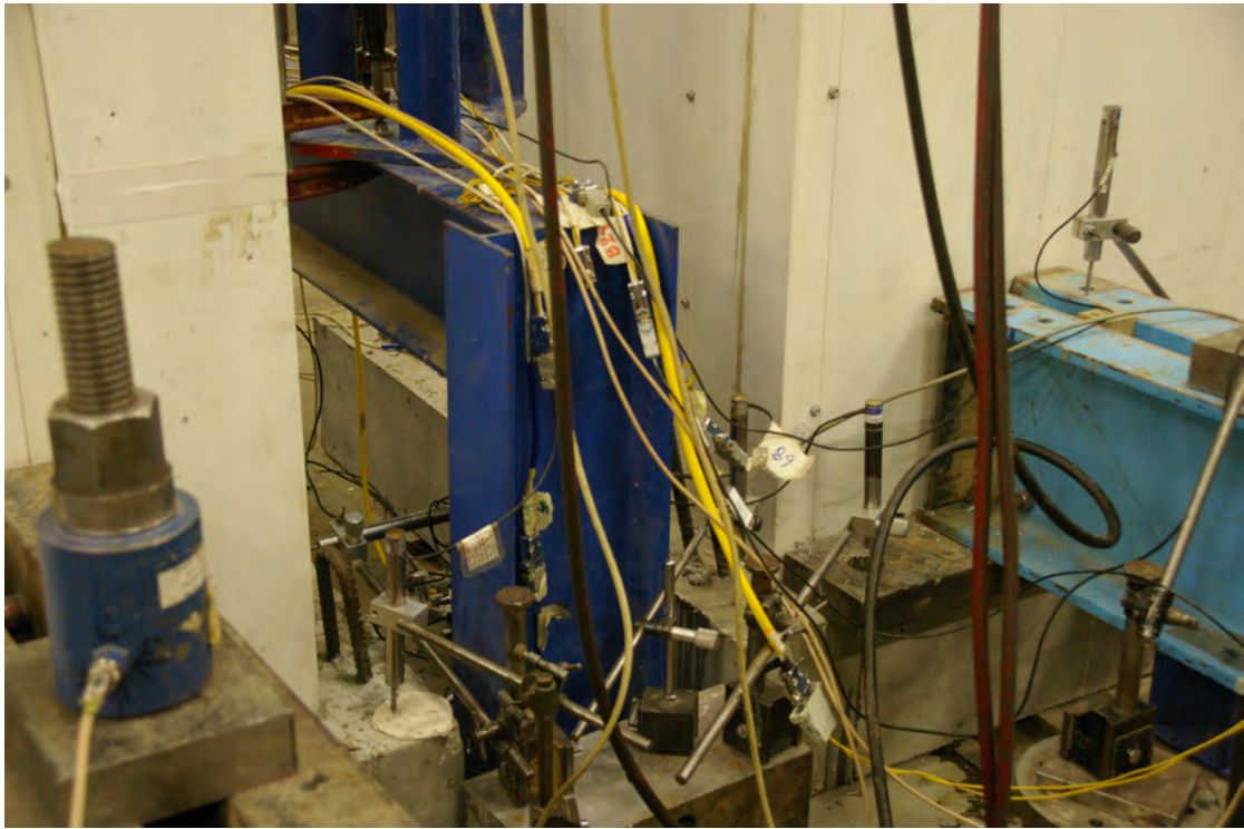
Figure 4.7 – bases of two Dintel walls on UTS strong floor ready for push over testing
