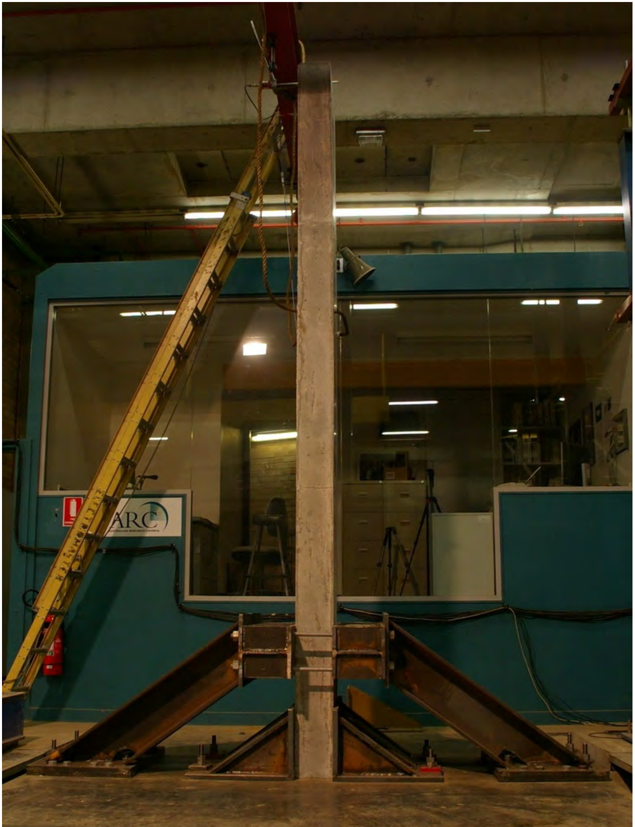
Fig 5.5 - Test set up on UTS Shake Table
