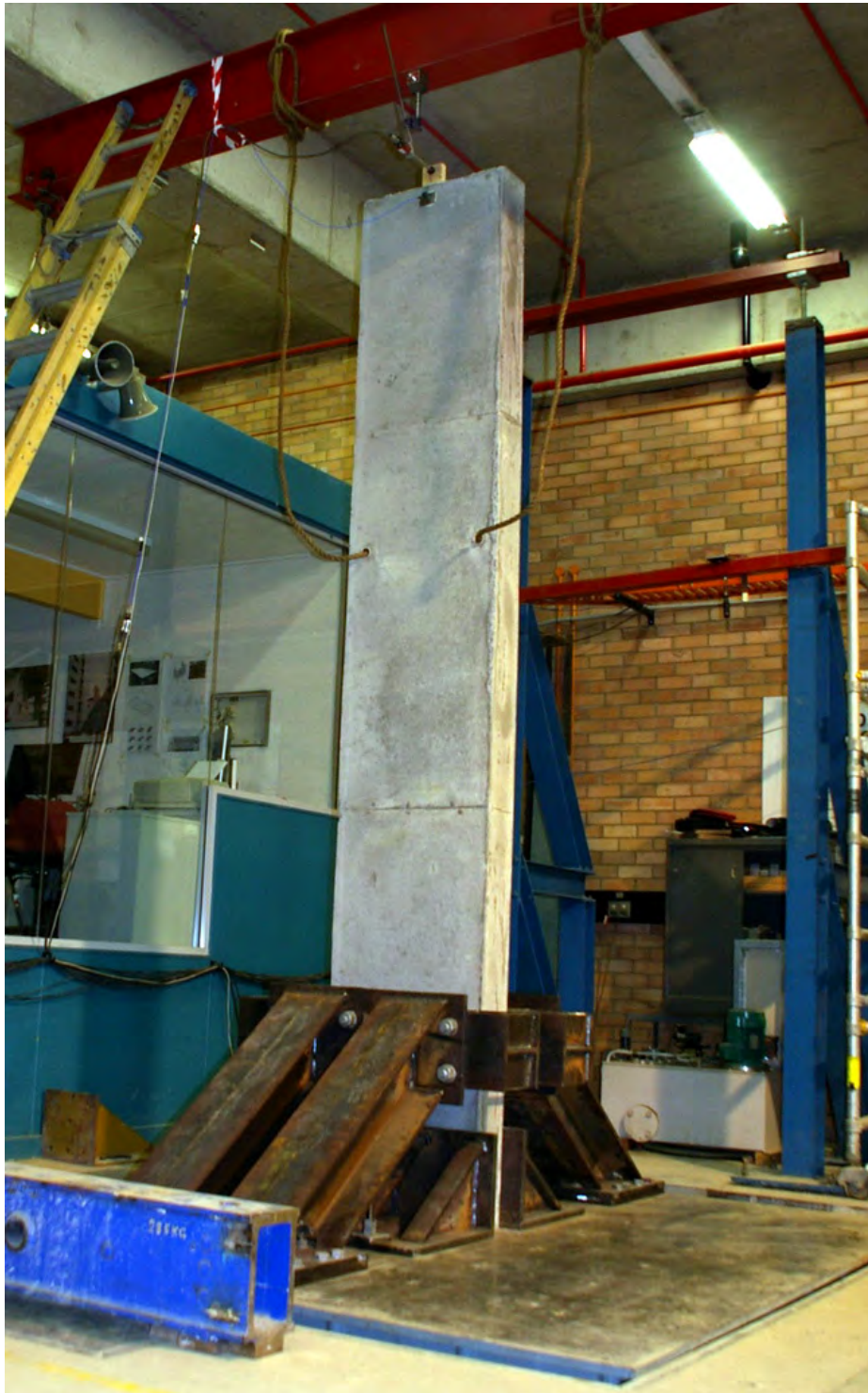
Fig 5.4- Conventional system Sample 'D' set up on UTS Shake Table
