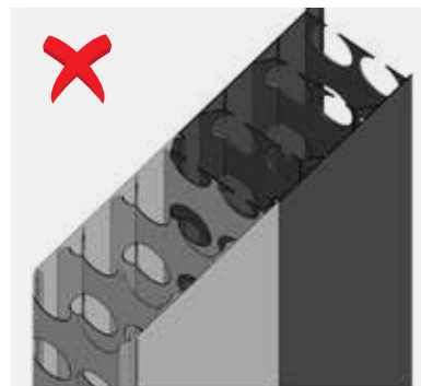
Incorrect – web holes do not align
