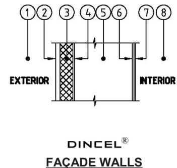
9. Minimum 25mm air gap between 6 & 7 if used additional R=0.16m<sup>2</sup> k/W can be added to the values shown above to achieve a higher rating. R = 2.01 + 0.16 = 2.17m<sup>2</sup> k/W for Option 2.
