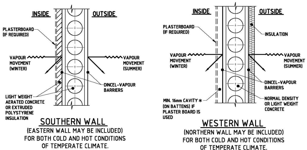
Both options should incorporate mechanical ventilation for bathrooms, laundries and kitchen exhausts, natural ventilation for the remaining areas. Western walls should incorporate shading on the walls and light coloured external paint finishes to reflect the sunlight for hot summer conditions.
