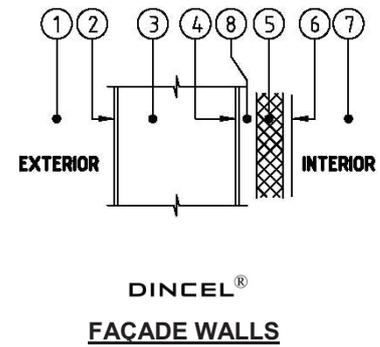
8. Minimum 25mm air gap between 4 & 5 or 6 if used additional R=0.16m<sup>2</sup> k/W can be added to the values shown above to achieve a higher rating, i.e. 28mm furring channels for internal plasterboard fixing achieves R = 1.95 + 0.16 = 2.11m<sup>2</sup> k/W for Option 2.
