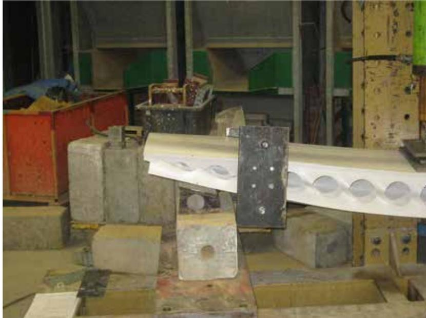
**Figure 75 – Hollow Dintel sample 2 at maximum loading**
