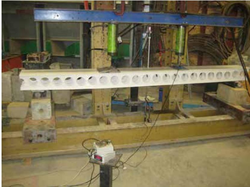
**Figure 79 – Hollow Dintel sample 3 after unloading**
