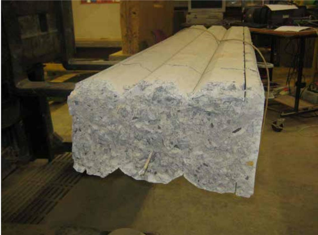
**Figure 44 – Conventional Reinforced Concrete sample 3 at failure cross section**
