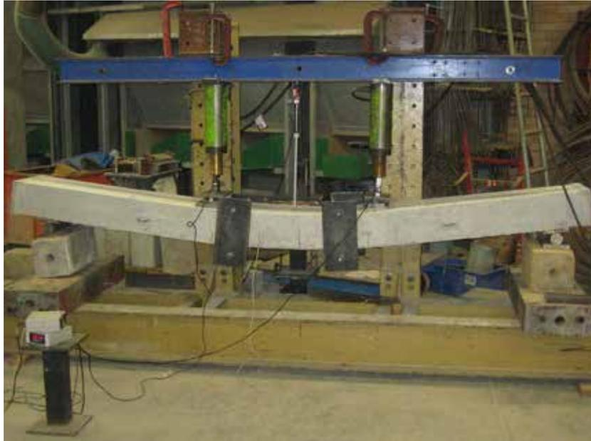
**Figure 51 – Reinforced Dintel sample during loading**
