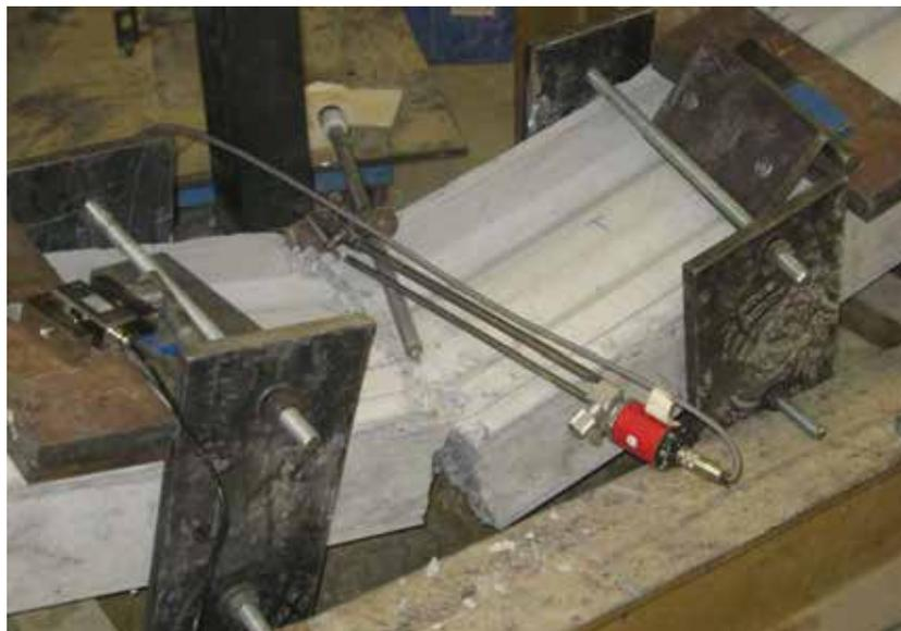
**Figure 43 – Conventional Reinforced Concrete sample 3 after failure**
