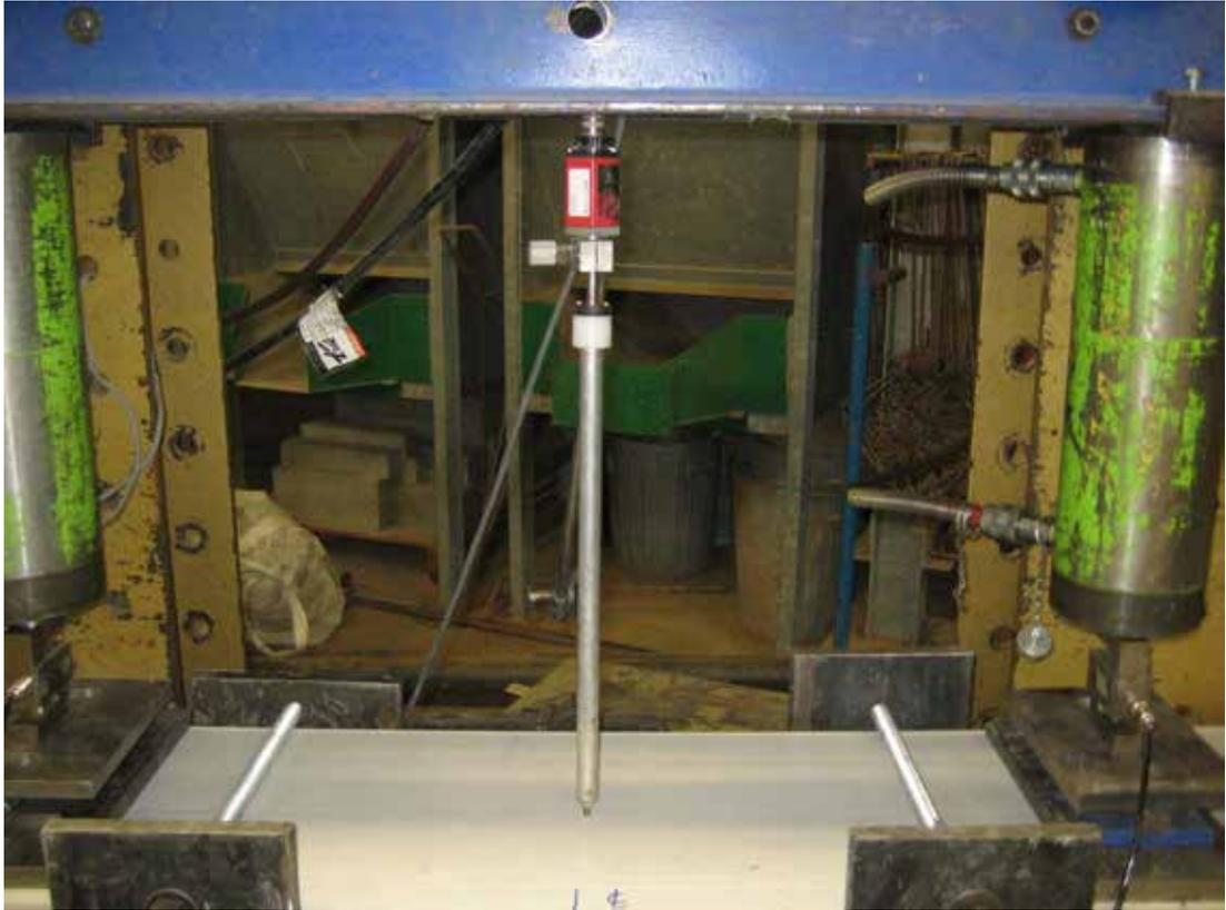
**Figure 28 – Linear variable displacement transducer (LVDT)**
