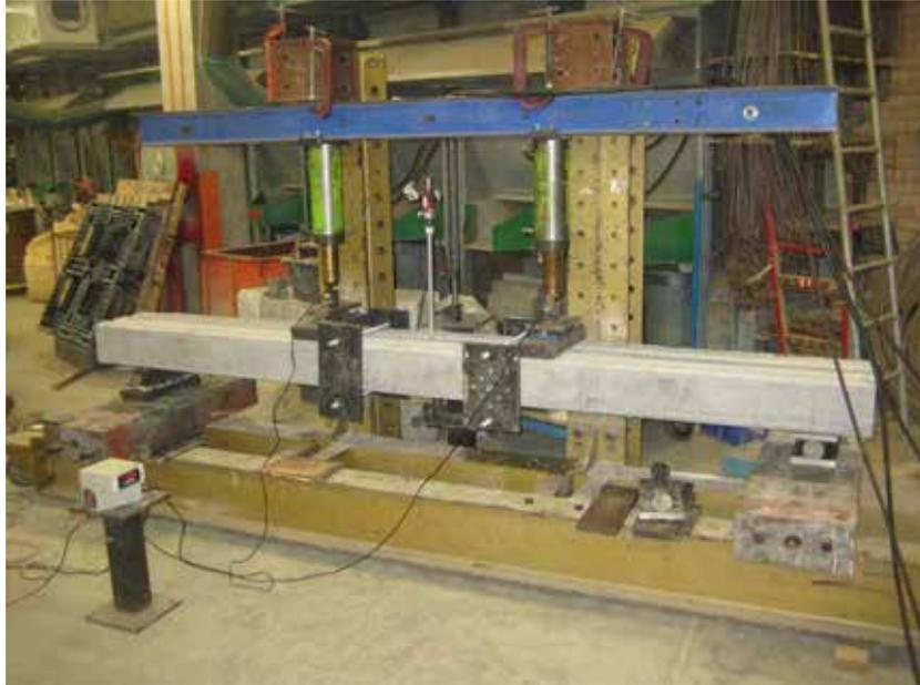
**Figure 38 – Conventional Reinforced Concrete sample ready for testing**
