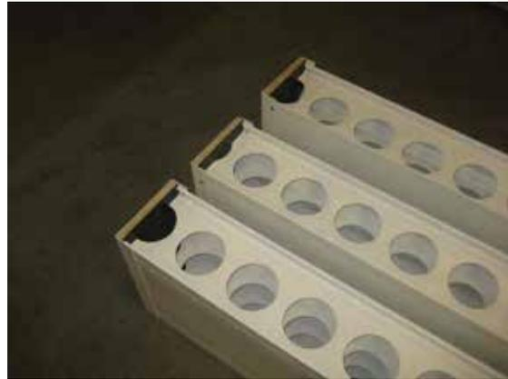
**Figure 20 – Unreinforced Dintel sample ends closed off**
