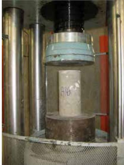
**Figure 35 – Sample compression testing**
