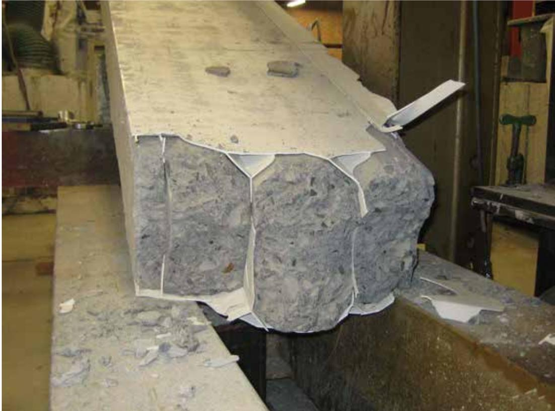
**Figure 63 – Cross section of Unreinforced Dincel sample 1 after failure**
