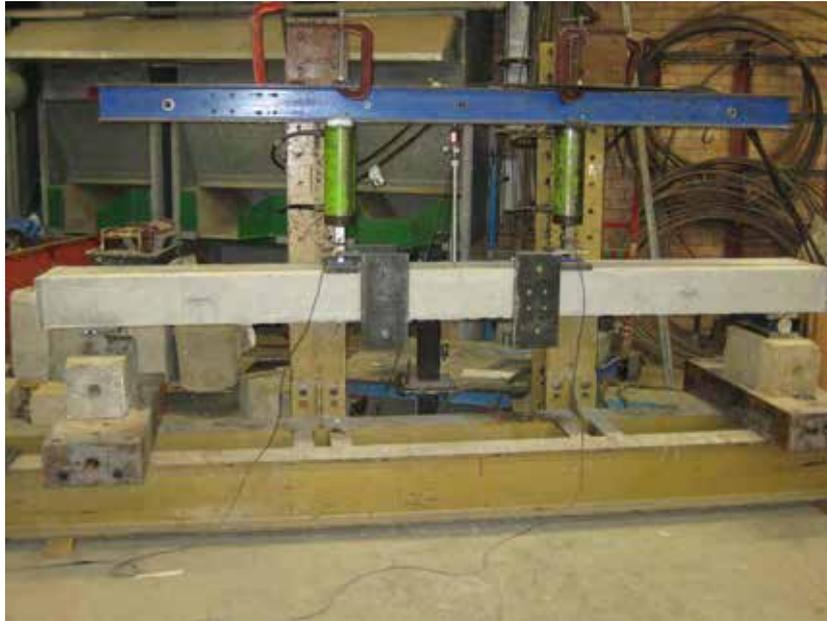
**Figure 60 – Unreinforced Dincel sample prior to loading**
