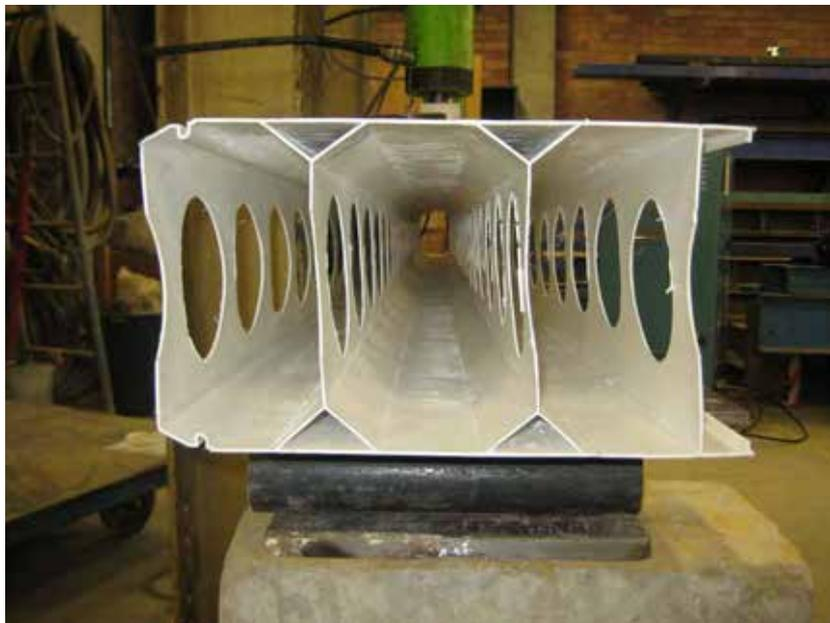
**Figure 70 – Hollow Dintel sample 1 prior to loading**
