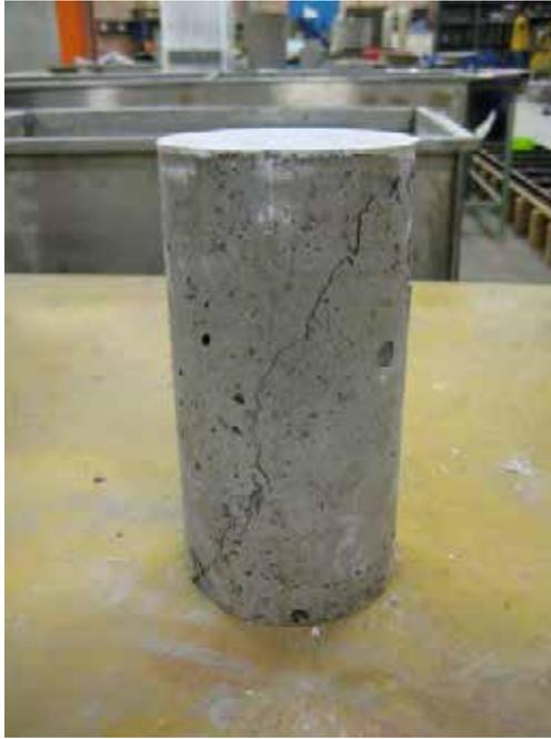
**Figure 37 – Concrete cylinder after failure**
