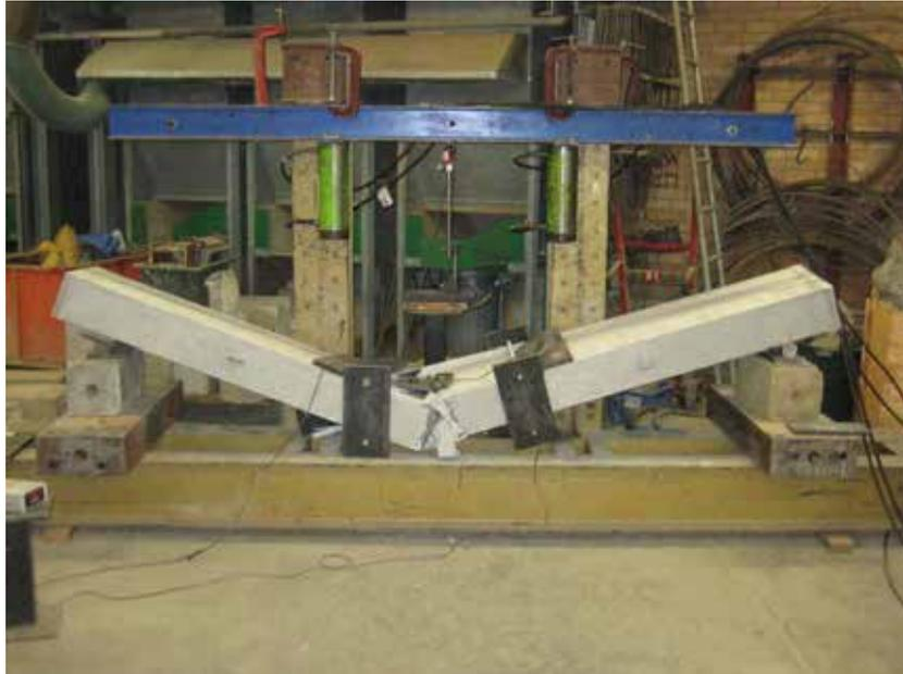
**Figure 62 – Unreinforced Dintel sample 1 tested to failure**
