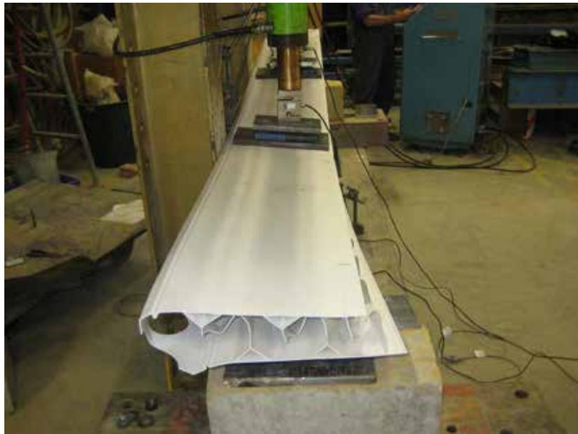
**Figure 78 – Hollow Dintel sample 3 during loading**
