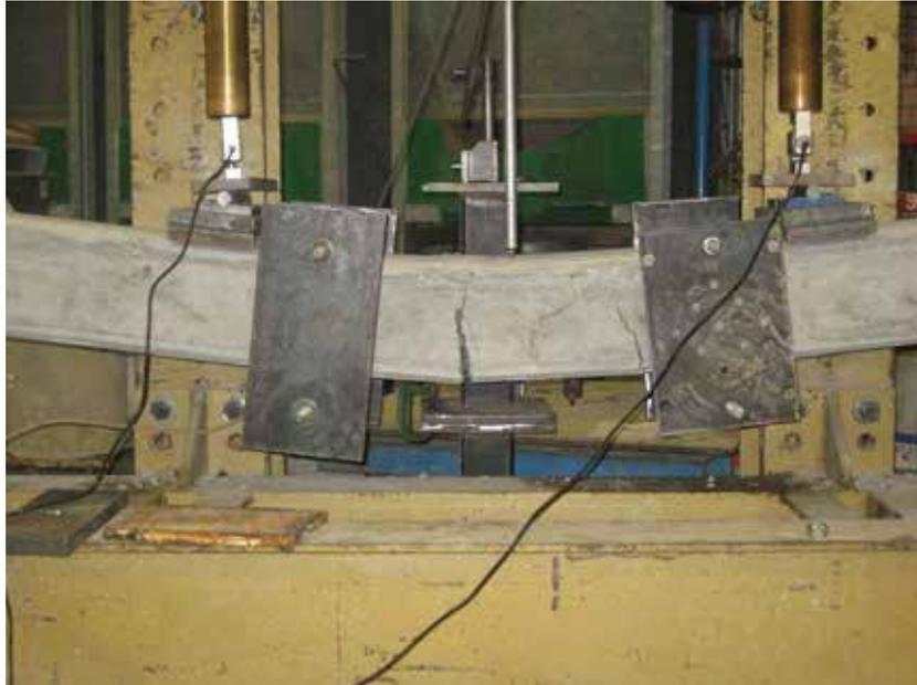
**Figure 42 – Large flexural cracks developing in Conventional Reinforced Concrete sample 3**
