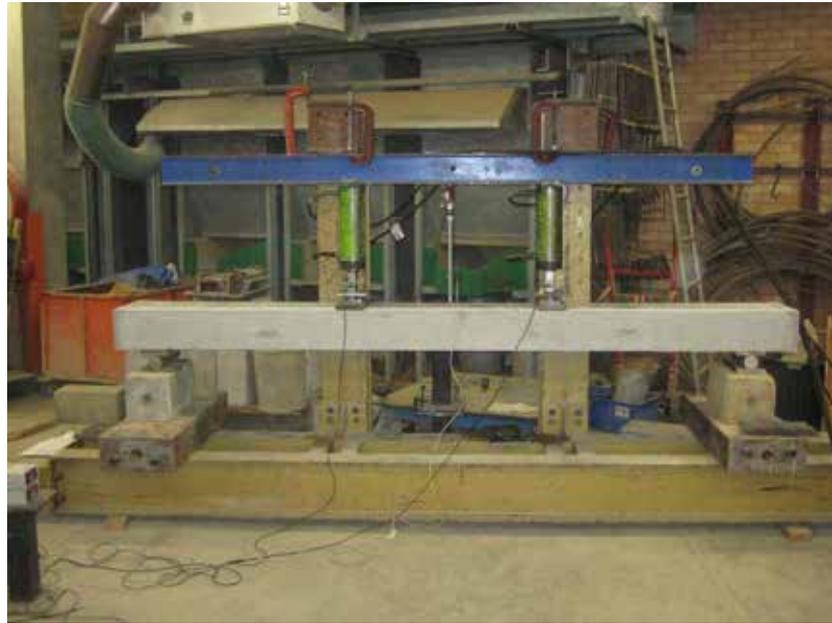
**Figure 49 – Reinforced Dintel Sample prior to loading**
