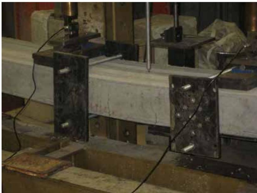
**Figure 39 – Flexural cracks in sample**
