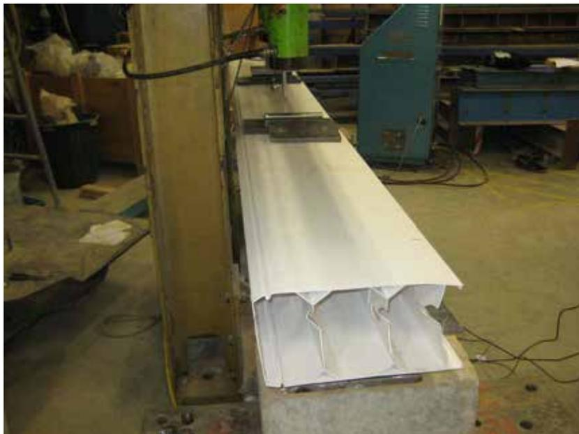
**Figure 80 – Hollow Dintel sample 3 after unloading**
