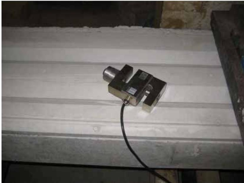
**Figure 26 – Load cell to be used during testing**
