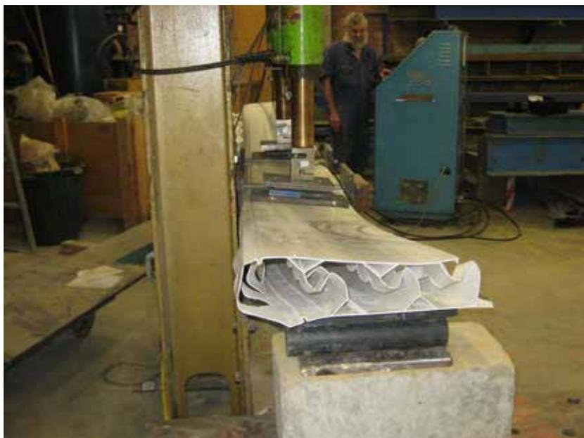
**Figure 72 – Hollow Dintel sample 1 at maximum loading**
