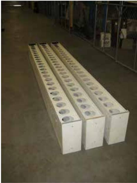
**Figure 19 – Unreinforced Dintel samples ready for concrete pouring**
