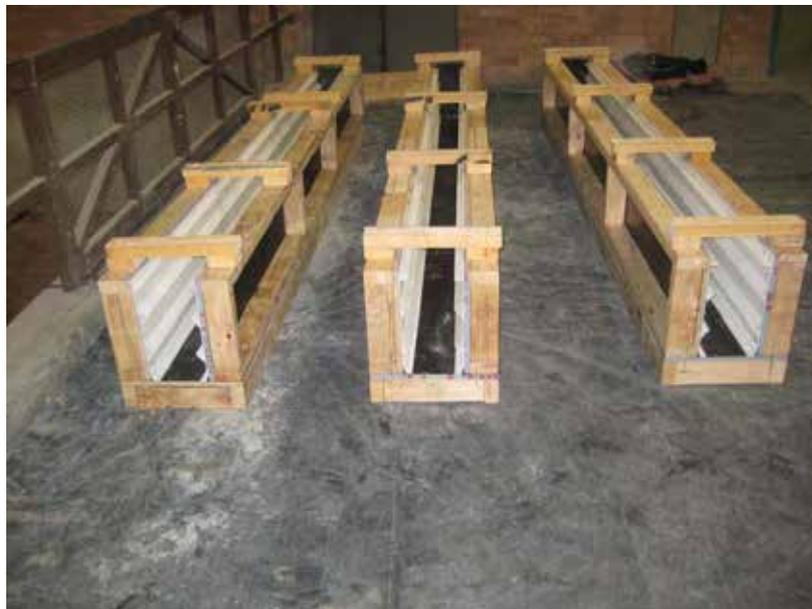
**Figure 10 – Cross-linking timber pieces**
