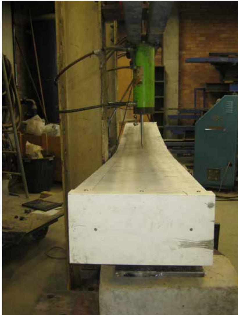
**Figure 53 – Deflection in Reinforced Dincel sample 1 after unloading**
