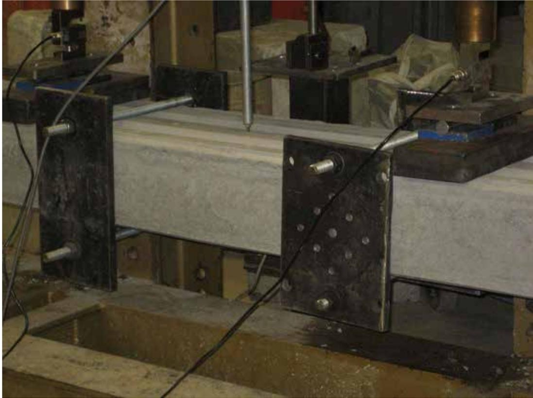
**Figure 27 – Steel plates used during testing**
