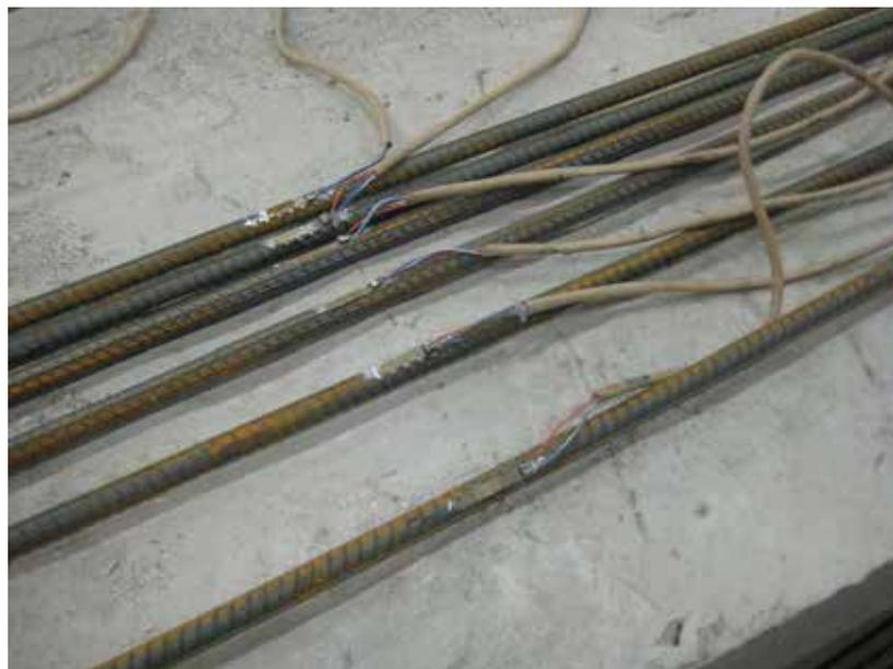
**Figure 1 - Attached strain gauges and two thin leads of each strain gauge**
