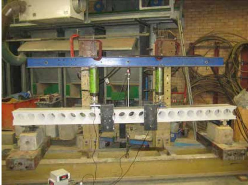
**Figure 69 – Hollow Dintel sample 1 prior to loading**
