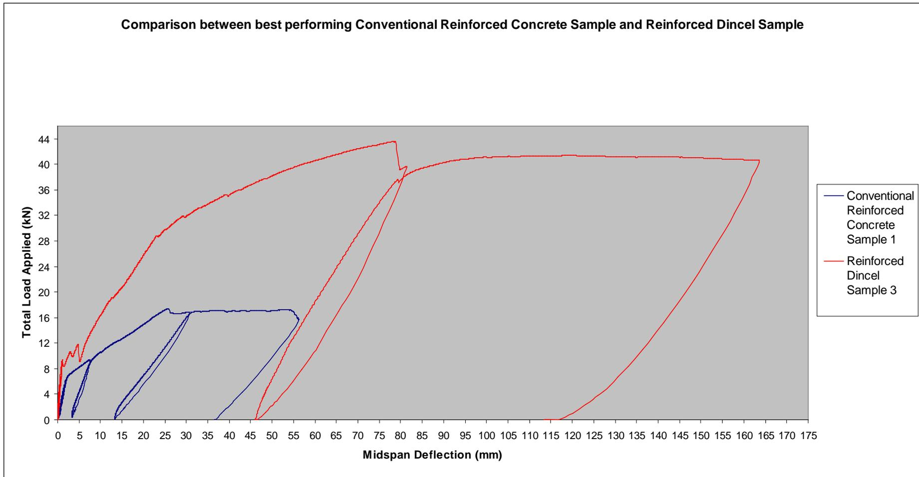
**Figure 59 - Total applied load vs midspan deflection comparison between the Conventional Reinforced Concrete sample which withstood the largest load (sample 1) and the Reinforced Dincel sample which withstood the largest load (sample 3)**
