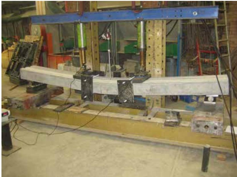
**Figure 41 - Conventional Reinforced Concrete sample during testing**
