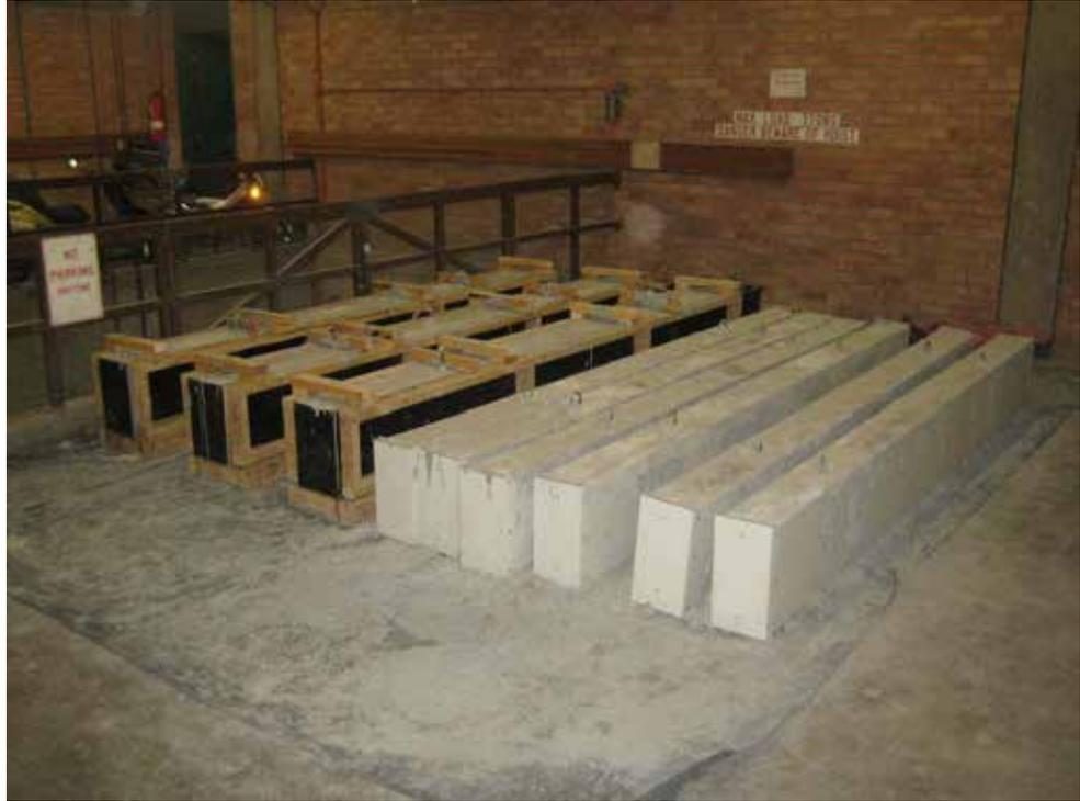
**Figure 24 – Testing samples after concrete pouring**
