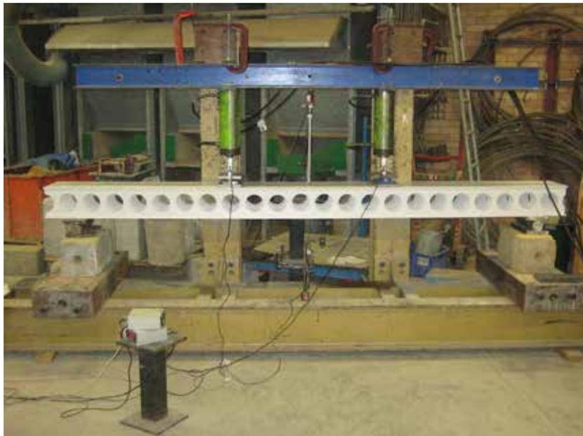
**Figure 76 – Hollow Dintel sample 3 prior to loading**
