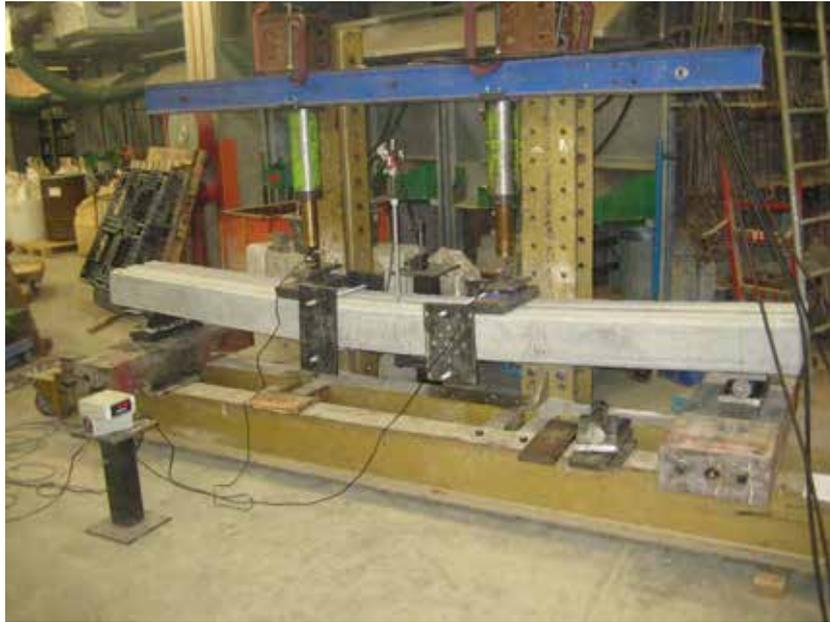
**Figure 40 – Conventional Reinforced Concrete sample during testing**
