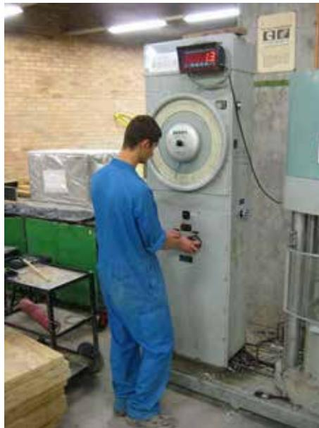
**Figure 36 – Operation of compression test machinery**
