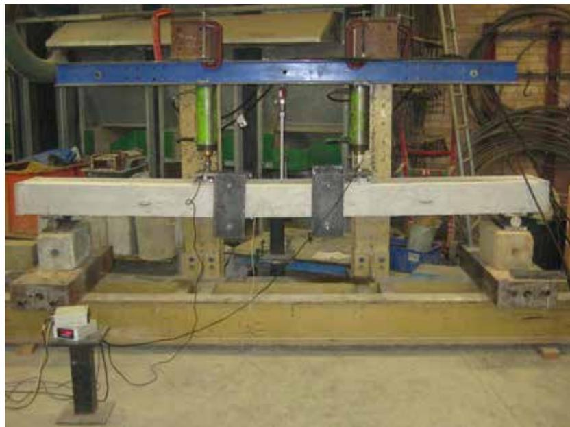
**Figure 50 – Reinforced Dintel sample during loading**
