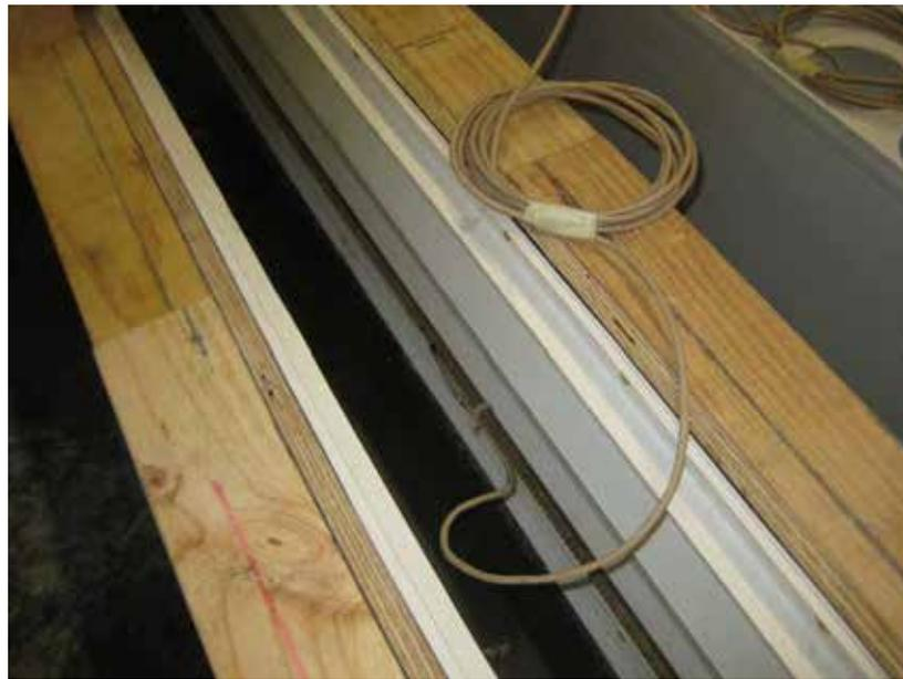
**Figure 13 – Cable attached to strain gauge**
